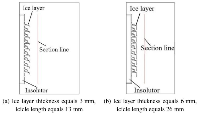
Fig. 2. Two-dimensional model of vertical icing insulator
