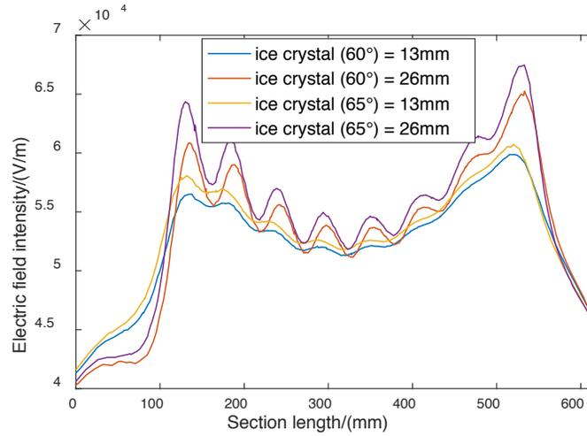
Fig. 5. Spatial electric field distribution of insulators with different arrangement angles of inclined cantilever
