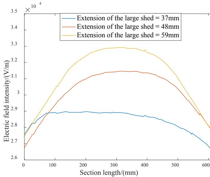
Fig. 8. Electric field distribution of icing insulators with different extension differences of the shed
