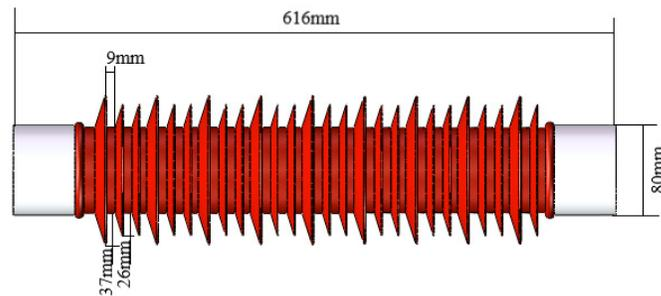
Fig. 9. Structure diagram of optimized insulator
