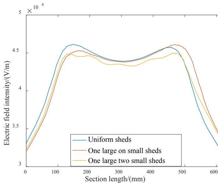
Fig. 6. Electric field distribution of icing insulators with different shed structures
