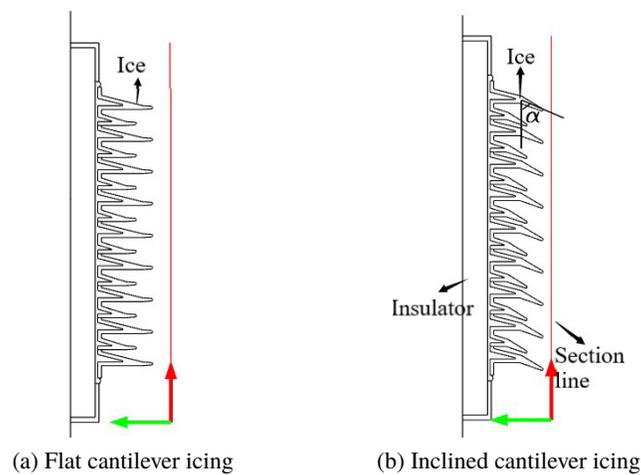
Fig. 3. Two-dimensional cantilever icing insulators
