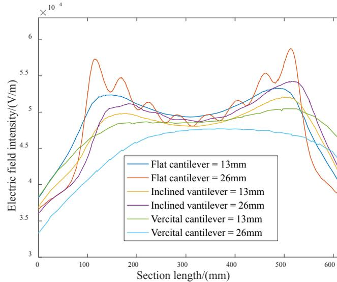
Fig. 4. Electric field distribution of insulators in different layout
