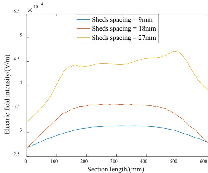
Fig. 7. Electric field distribution of icing insulators with different shed spacing
