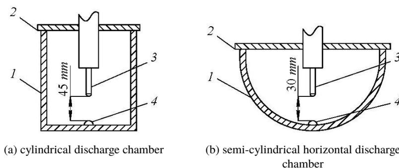
Fig. 1. Scheme of electric discharge chambers: 1 – chamber body; 2 – lid; 3 – high voltage electrode; 4 – grounded electrode
