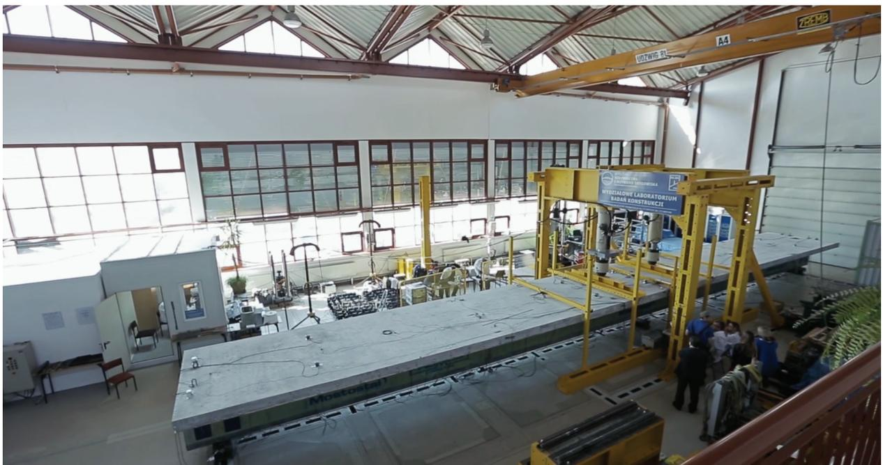
Fig. 3. Full scale laboratory tests of FRP road bridge at Rzeszow University of Technology [24]
