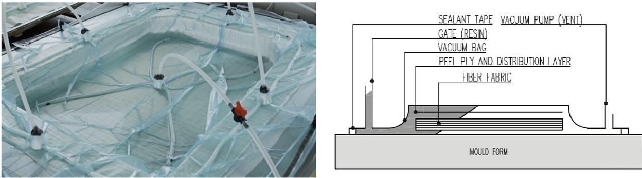
Fig. 1. VARTM process in Mostostal Warszawa [24] and the general scheme of VARTM production method [4]
