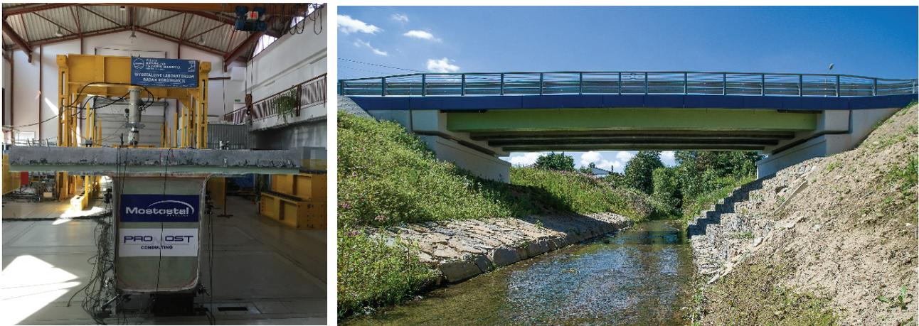
Fig. 13. Bridge in Błażowa nearby Rzeszów – single girder tests at Rzeszow University of Technology and side view of the bridge [16]
