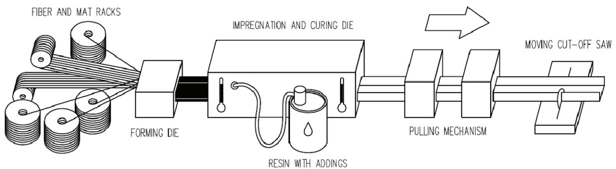
Fig. 2. Pultrusion process scheme [7]
