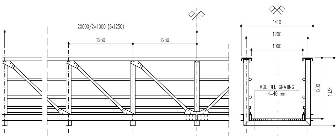
Fig. 5. Longitudinal and cross section of the pedestrian truss bridge [18]
