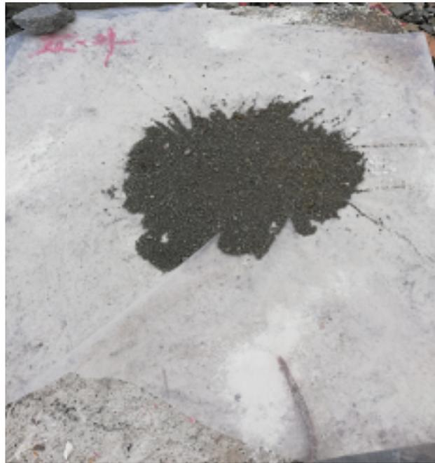
Fig. 8. Measuring the blasted Volume
