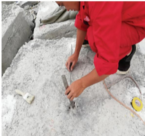
Fig. 5. Measuring the Cutting depths
