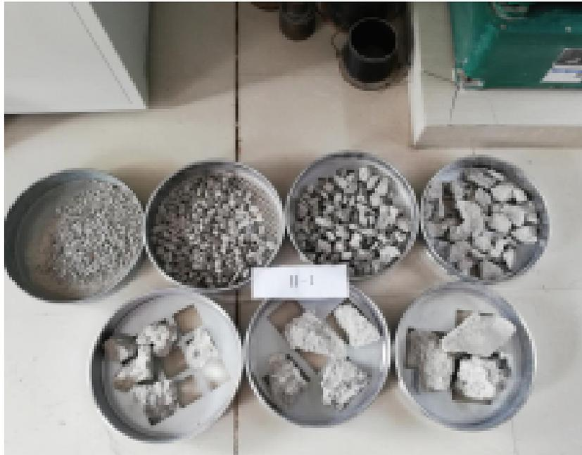
Fig. 12. Blasting fragmentation screening
