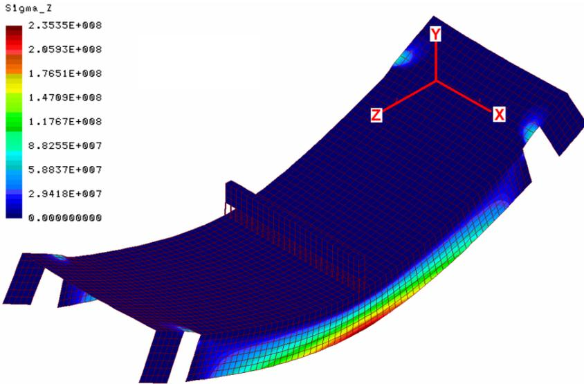
Fig. 25. Distribution of tensile stress in the Z direction (stress in Pa, deformation scale 10 $\times$ )
