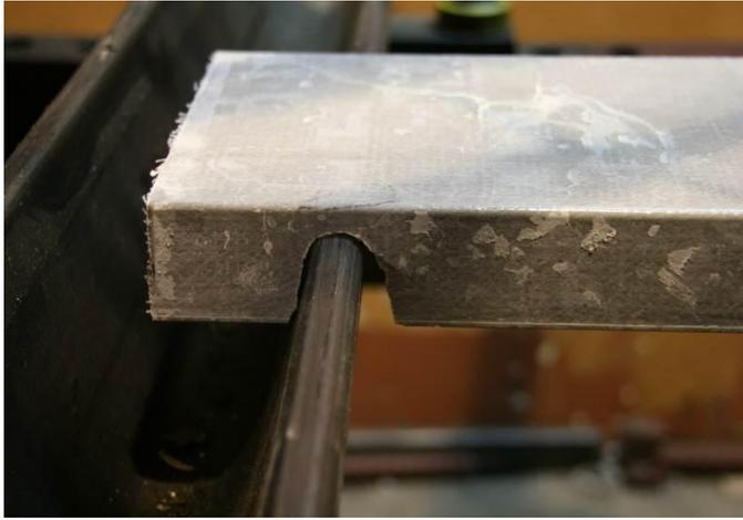
Fig. 6. Structural C-channel lining with a single gap
