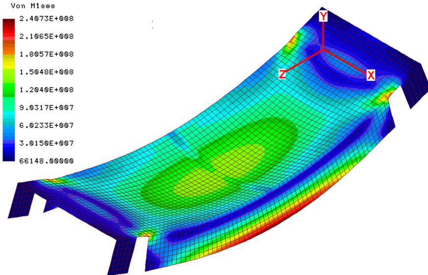
Fig. 26. Von Misses stresses for maximum loads (stress in Pa, deformation scale 5 $\times$ )
