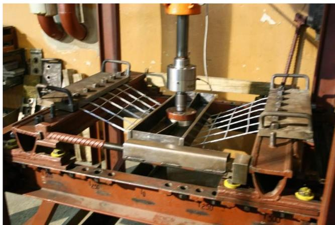
Fig. 10. Method of testing lining meshes
