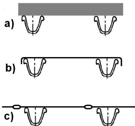
Fig. 9. Various technical solutions for mining linings
