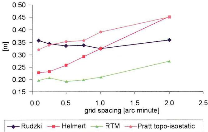
Fig. 12. Standard deviation of the differences between different geoid undulations with GPS/levelling geoid before fit
