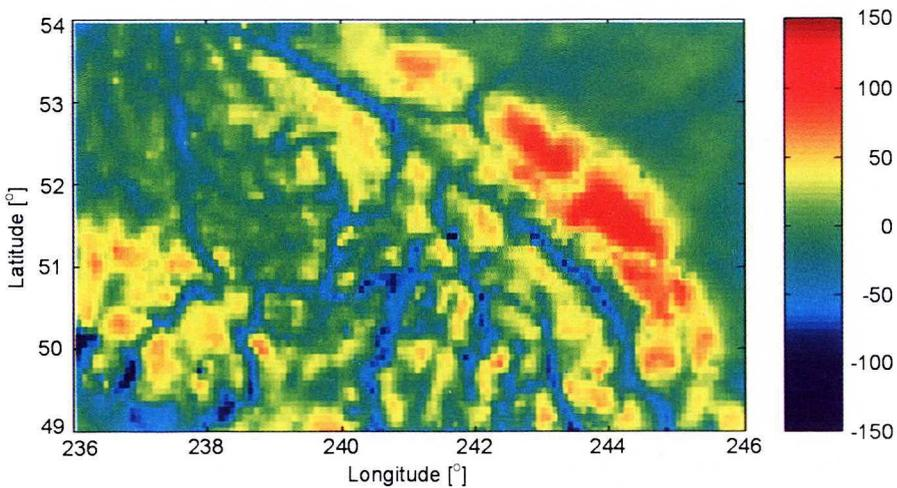
Fig. 6. 6''x6'' Ruzzki anomalies using 6'' DTM grid resolution [mGal]
