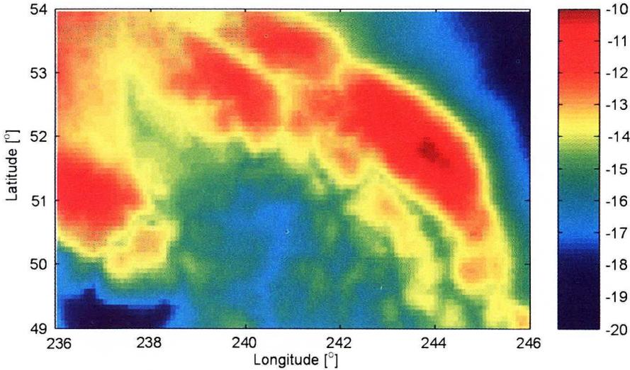
Fig. 11. 5' × 5' Rudzki geoid using 2' DTM grid resolution [m]
