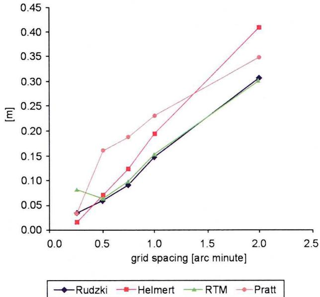
Fig. 9. The difference in standard deviation between the control geoid and the geoid models obtained using different DTM resolutions
