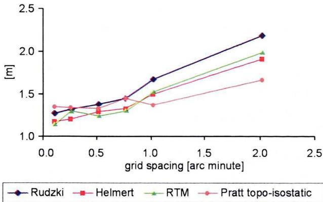
Fig. 14. The range of differences between different geoid undulations with the GPS/levelling geoid after fit
