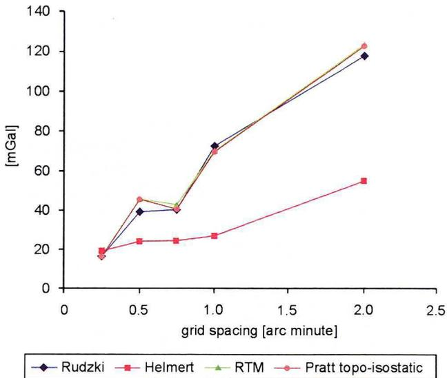
Fig. 4. The difference in maximum value between control gravity anomalies and anomalies obtained using different DTM resolutions
