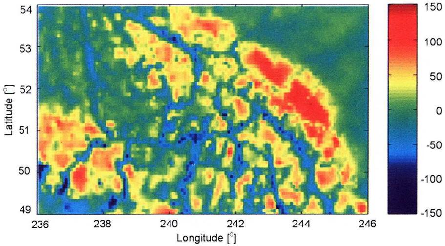
Fig. 7.  $5' \times 5'$  Rudzki anomalies using  $2'$  DTM grid resolution [mGal]
