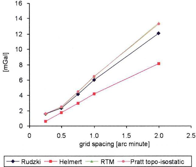
Fig. 5. The difference in standard deviation between control gravity anomalies and anomalies obtained using different DTM grid resolutions
