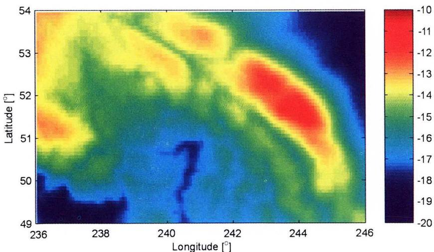
Fig. 10.  $6'' \times 6''$  Ruzdki geoid using  $6''$  DTM grid resolution [m]
