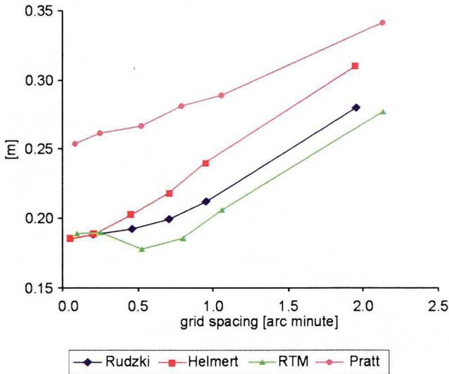
Fig. 13. Standard deviation of the differences between different geoid undulations with the GPS/levelling geoid after fit
