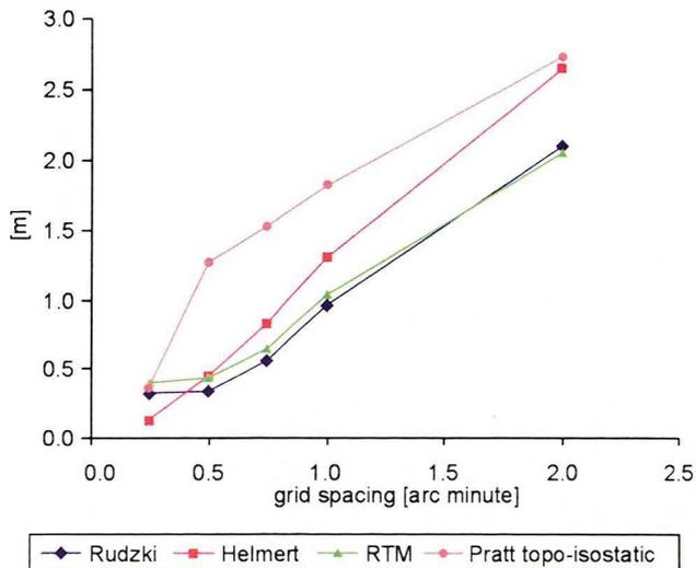
Fig. 8. The difference in maximum value between the control geoid and geoid models obtained using different DTM resolutions
