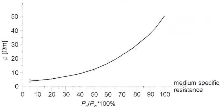
Fig. 2. Diagram of relations of power of recorded impulses of electromagnetic waves and the medium specific resistance
