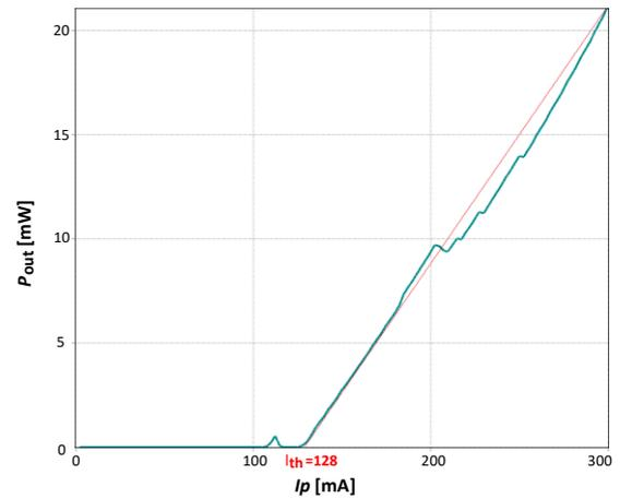
Fig. 14. BD2 threshold current ( $I_{th}$ ).
