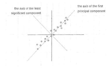
Fig. 4. The direction of the greatest and the smallest variance of input data determined by principal components
