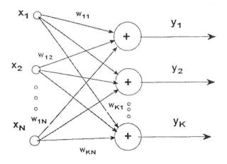
Fig. 2. A unidirectional neuron network for data compression
