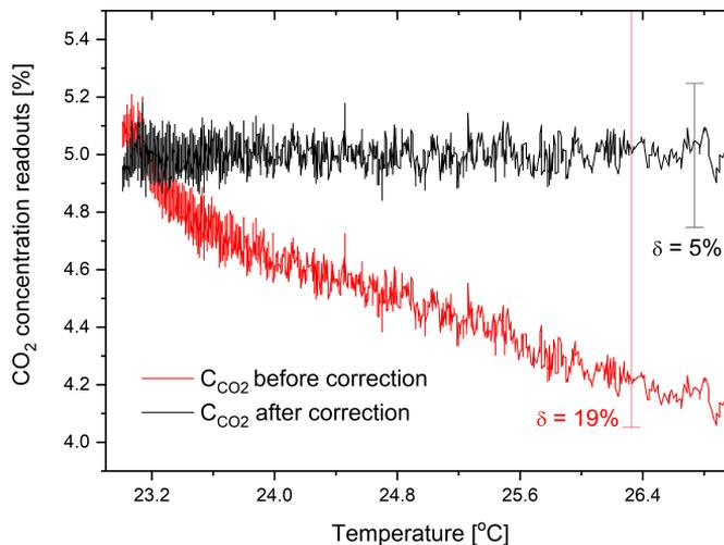
Fig. 7. Temperature influence on UT100C CO<sub>2</sub> sensor readouts before and after correction.
