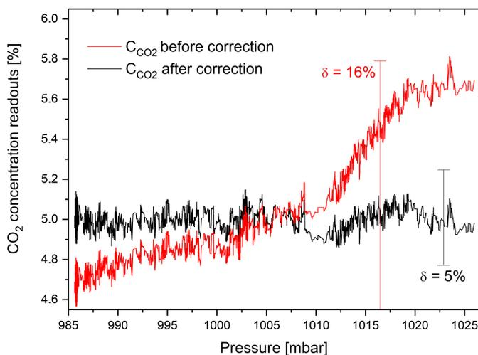
Fig. 6. Pressure influence on the UT100C CO<sub>2</sub> sensor readouts before and after correction.
