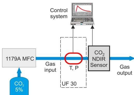
Fig. 5. Experimental setup for testing the CO<sub>2</sub> sensor.
