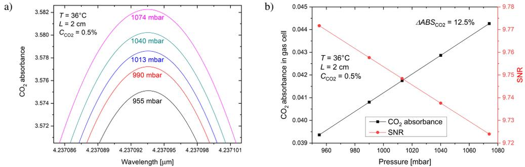
Fig. 3. CO<sub>2</sub> absorbance changes on the selected gas absorption line (a), CO<sub>2</sub> absorbance in the gas cell and SNR as a function of human exhaled air pressure (b).
