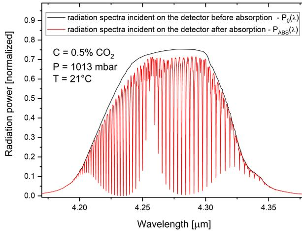
Fig. 2. Spectrum of LED radiation after passing through the empty (black line) and the breath-filled gas cell (red line).
