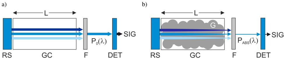
Fig. 1. Components of the NDIR sensor:  $P_0(\lambda)$  is the radiation power incident on the detector with absence of gas in the gas cell (a),  $P_{ABS}(\lambda)$  is the radiation power incident on the detector when the test gas is present in the gas cell (b).
