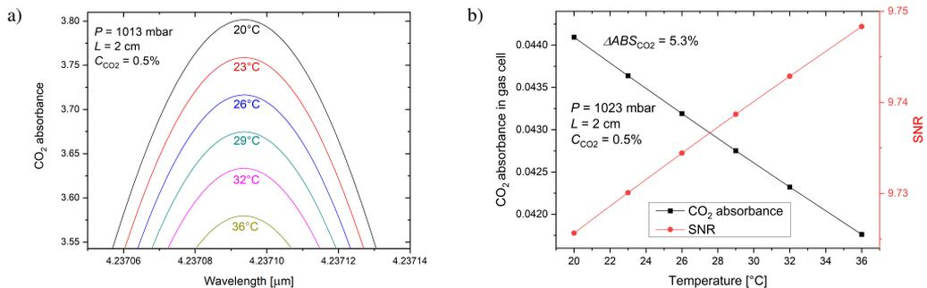
Fig. 4. CO<sub>2</sub> absorbance changes on the selected gas absorption line (a), CO<sub>2</sub> absorbance in the gas cell and SNR as a function of human exhaled air temperature (b).
