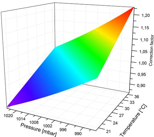
Fig. 8. Correction factors for pressure and temperature influence on CO<sub>2</sub> sensor measurements.
