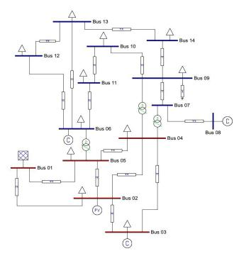
Fig. 3. IEEE 14-bus system's PSAT model
