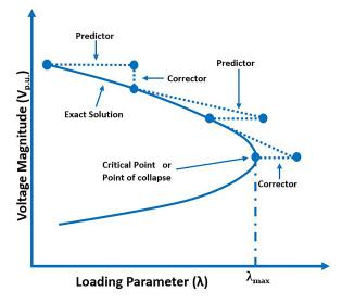
Fig. 2. Predictor-corrector approach used in the CPF
