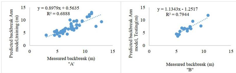
Fig. 9. Correlation of the measured back break with the predicted back break ANN model (A: Training), and (B: Testing)
