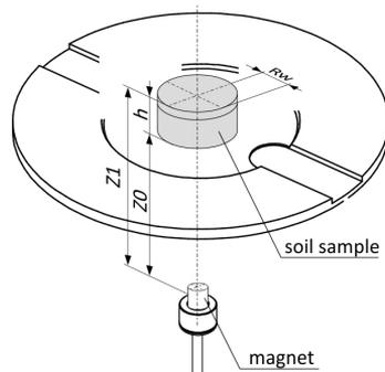
Fig. 3. Dimensions of the measuring system.  $Z_0$  – distance from the center of the magnet to the bottom of the sample,  $Z_1$  – distance from the top of sample to the center of the magnet,  $h$  – sample height,  $R_w$  – radius of the soil sample.
