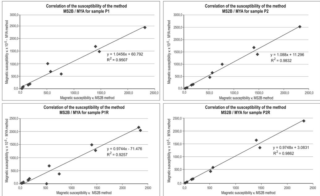
Fig. 9. Correlation between measurements of  $\kappa$  values using the MS2B Bartington sensor and the MYA weighting method.
