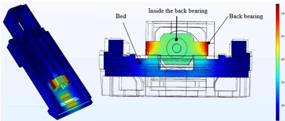
Fig. 7. Predicted temperature distribution on the structure
