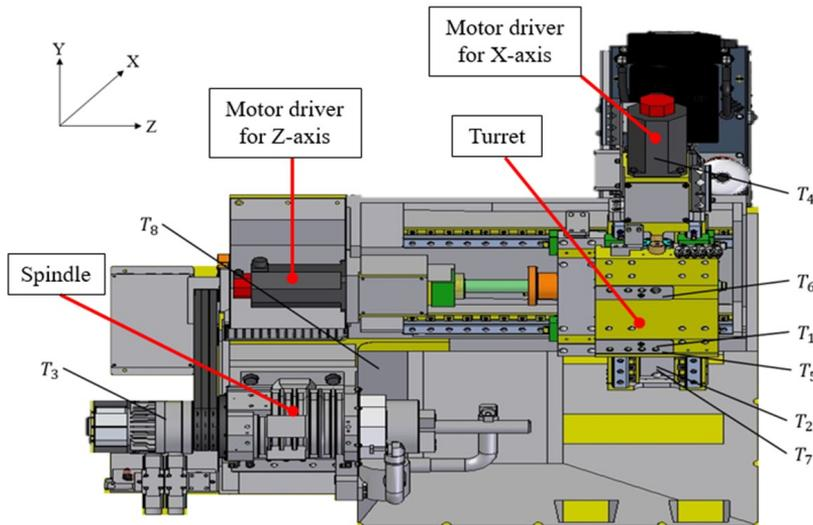
Fig. 1. Experimental machine tool and locations of thermocouples
