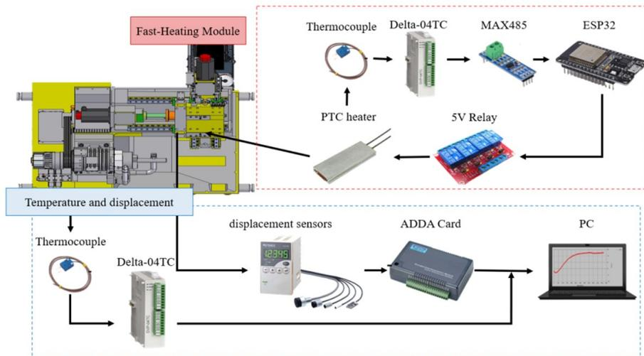
Fig. 2. The whole experimental structure
