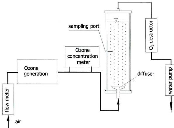
Fig. 1. Scheme of the laboratory test stand.
