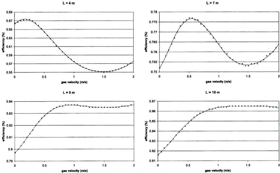
Fig. 6. The efficiency of the ESP in the middle of zone as a function of gas velocity ( $v_g$ ) for  $L = 4$  m,  $L = 7$  m,  $L = 9$  m and  $L = 10$  m
