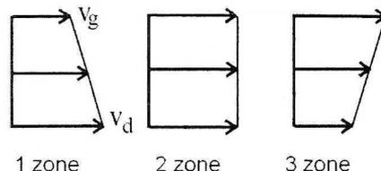
Fig. 1. Linear-skewed gas flow profile by Hein
