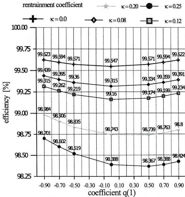
Fig. 4. Efficiency of ESP as a function of skew-coefficient
