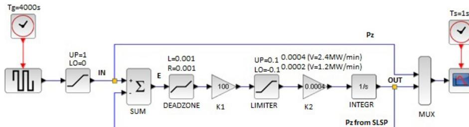
Figure 3: Scheme of the speed limiter of set power (SLSP):  $T_g$  – initialization time of the clock,  $T_s$  – period of the clock,  $V$  – speed setting of setpower,  $L$  – lower (left) limit of deadband,  $R$  – upper (right) limit of deadband,  $UP$  – upper limit of saturation,  $LO$  – lower limit of saturation,  $P_z$  – setpower. Other markings in the text.
