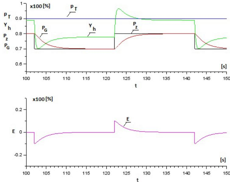
Figure 7: Simulation of manual power control of the turboset:  $p_T$  – pressure of the steam from the boiler,  $P_z$  – set power,  $P_G$  – generator (real) power,  $Y_h$  – position of the control valve (inlet signal of the power generator),  $E$  – deviation of control signal. Optimal settings of the controller PI ( $K_p = 2$ ,  $T_i = 0.4$ ).
