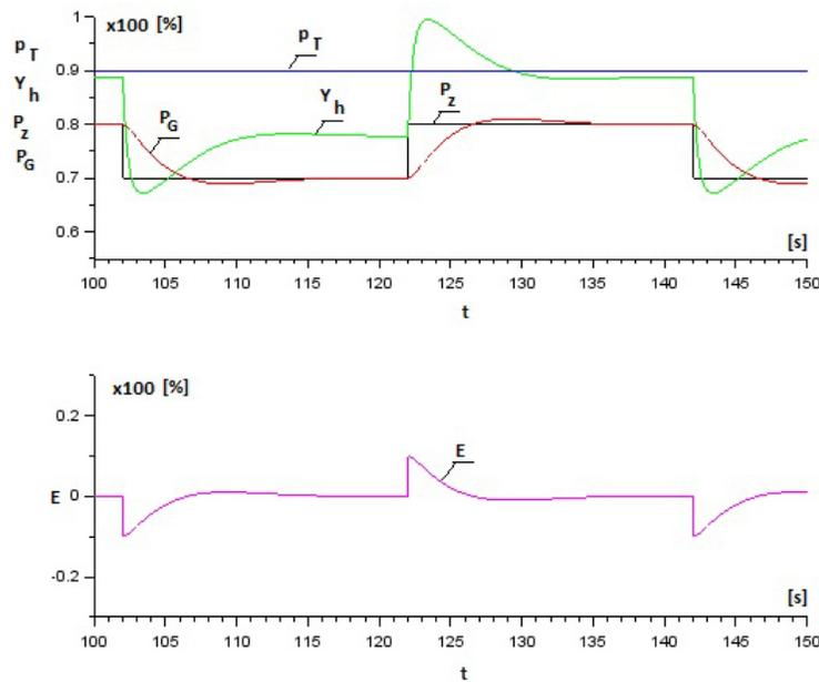
Figure 12: Simulation of power control of the turboset. Settings of the controller PI:  $K_p = 2$ ,  $T_i = 0.8$ .
