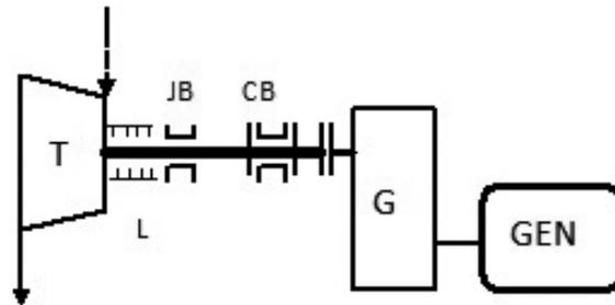
Figure 1: Schematic view of the turbine [6]: T – turbine, L – labyrinth seal, G – gear, GEN – generator, JB – journal bearing, CB – combined (thrust/journal) bearing.
