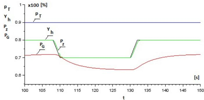
Figure 13: Simulation of manual power control of the turboset at a linear increase in the set signal.
