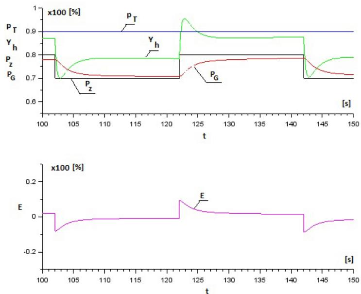
Figure 9: Simulation of power control of the turboset. Settings of the controller PI:
