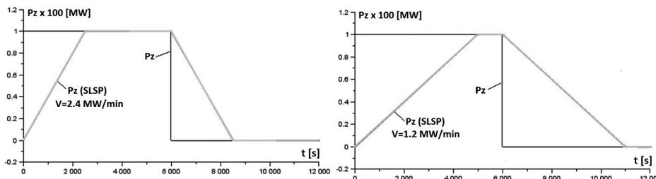
Figure 4: The speed limiter of setpower response to the speed  $V = 1.2$  MW/min and  $2.4$  MW/min; setpower  $100$  MW ( $y$ -axis) changes in  $5000$  s (for  $V = 1.2$  MW/min) or in  $2500$  s (for  $V = 2.4$  MW/min).
