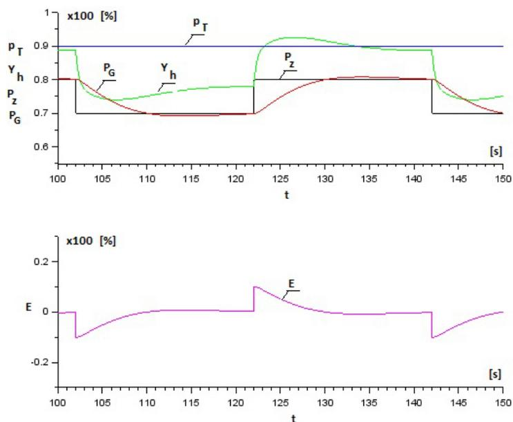
Figure 8: Simulation of power control of the turboset. Settings of the controller PI:
