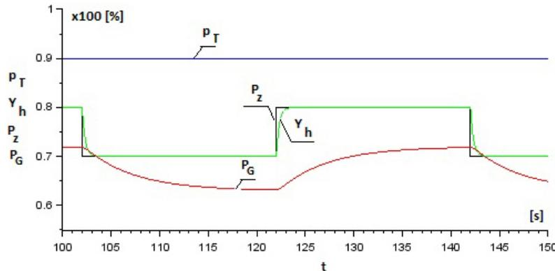
Figure 6: Simulation of manual power control of the turboset:  $p_T$  – pressure of the steam from the boiler,  $P_z$  – set (real) power,  $P_G$  – generator power (real),  $Y_h$  – position of the control valve.
