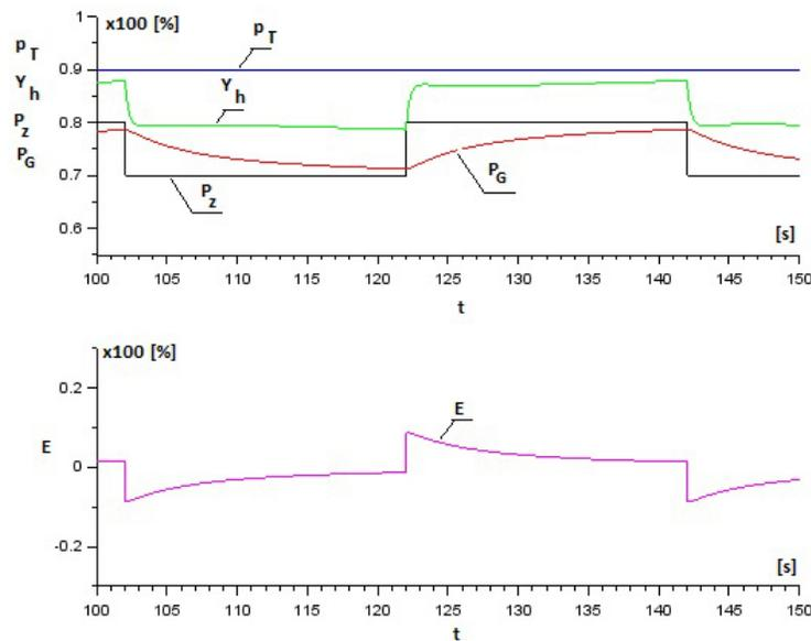
Figure 10: Simulation of power control of the turboset. Settings of the controller PI:  $K_p = 1$ ,  $T_i = 0.1$ .
