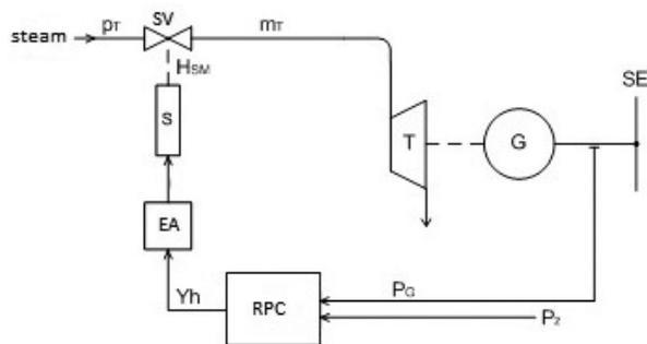
Figure 5: Technological scheme (part) of the power generation turboset:  $p_T$  – pressure of the steam from the boiler, SV – steam valve,  $H_{SM}$  – leap (displacement) of the servomotor spindle,  $m_T$  – steam mass flow rate, T – steam turbine, S – servomotor, EA – electrohydraulic actuator,  $Y_h$  – set-up signal, RPC – real power controller,  $P_G$  – real power generated by the generator G,  $P_Z$  – set (real) power, SE – electricity generation system.
