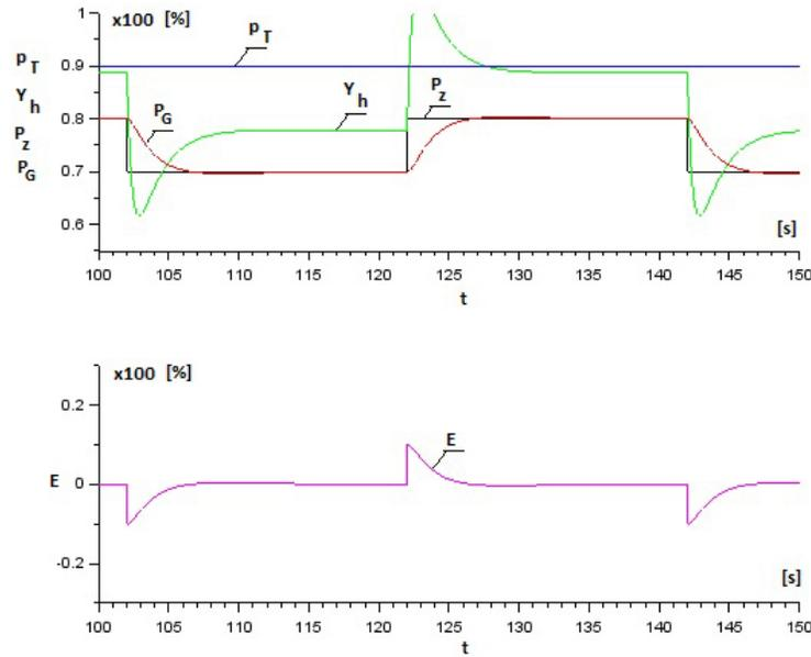
Figure 11: Simulation of power control of the turboset. Settings of the controller PI:  $K_p = 3$ ,  $T_i = 0.8$ .
