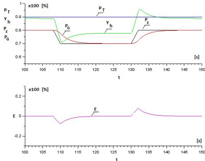
Figure 14: Simulation of power control of the turboset at a linear increase in the set power signal. Optimal settings of the controller PI ( $K_p = 2$ ,  $T_i = 0.4$ ).
