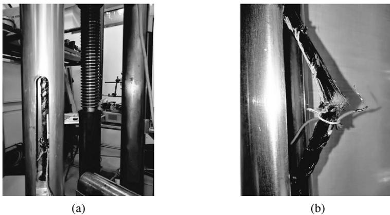
Fig. 2. (a) Device for testing the BFRP reinforcing bars, (b) BFRP sample with free unbraced length of  $26d_b$  damaged due to buckling
