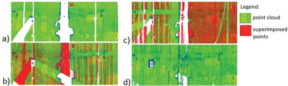
Fig. 3. Fragments of point clouds: a) ST7, b) ST7 with superimposed points from ST6, c) ST7 with superimposed points from ST8, d) ST7 with superimposed points from ST6 and ST8 (own elaboration)
