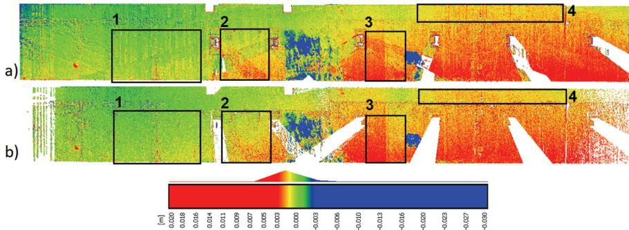
Fig. 7. Differential model of the investigated surface (distances determined with M3C2 algorithm) based on data from cycle 1 and cycle 2: a) point clouds subjected only to filtration, b) with application of point clouds limiting criteria proposed in the methodology. Black boxes (from 1 to 4) mark the areas of the most significant differences in obtained results (own elaboration)
