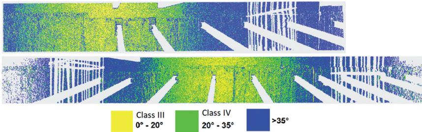
Fig. 5. Incidence angle distribution of the laser beam, ST3 and ST4 respectively
