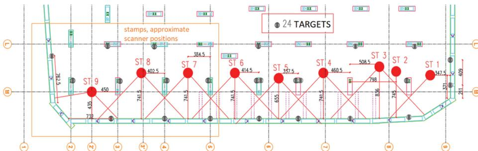
Fig. 2. Layout design of the scanner stations (ST1–ST9) and measurement targets for the selected slurry wall of the test facility
