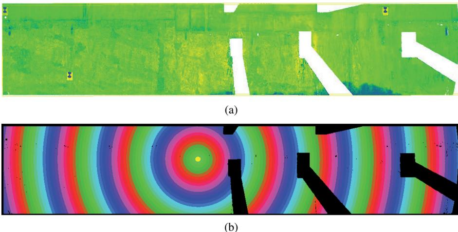
Fig. 4. Concentric nature of the distribution of the influences of the beam incidence angle and scanning distance on the recorded beam reflection intensity values: a) scan of the slurry wall in intensity colors, b) distribution of influences of geometrical factors (incidence angle, distance), a 10 cm step along the measured wall, centre: projection of the center point of the scan
