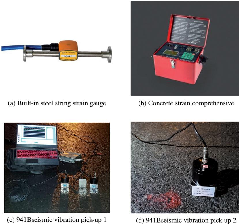
Fig. 4. Sensors used in the test
