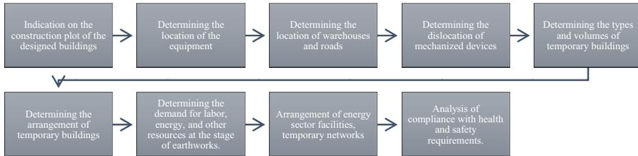
Fig. 7. Mathematical model of site construction for earthworks and concrete works
