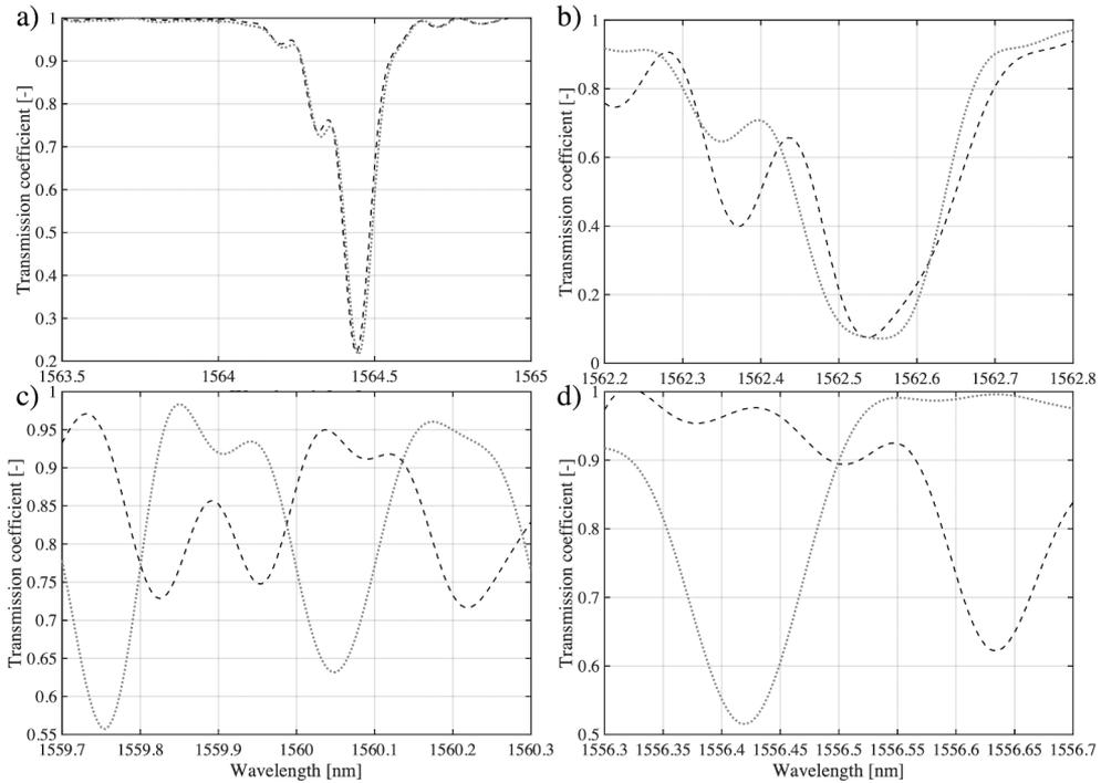
Fig. 5. Modifications of individual modes of the TFBG structure subjected to bending, Bragg resonance (a), ghost mode (b), LP<sub>110</sub> (c), and LP<sub>015</sub> (d).
