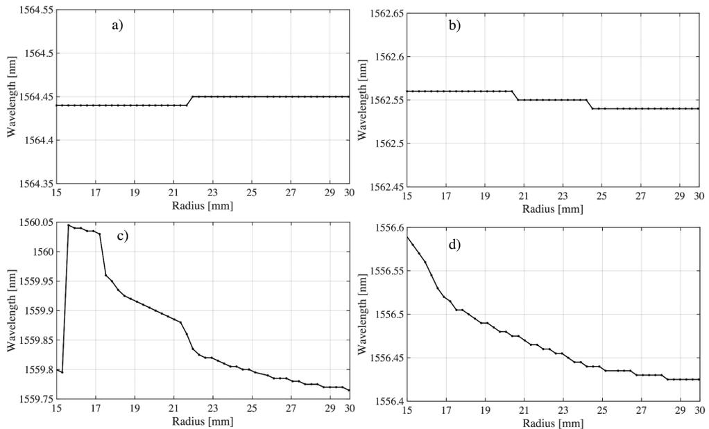
Fig. 6. Characteristics of TFBR processing when subjected to bending for selected propagating modes in the structure: Bragg resonance (a), ghost mode (b), LP<sub>110</sub> (c), and LP<sub>015</sub> (d).
