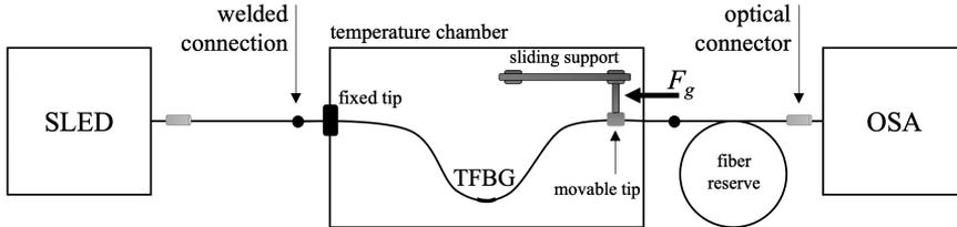
Fig. 2. Scheme of the measurement system.
