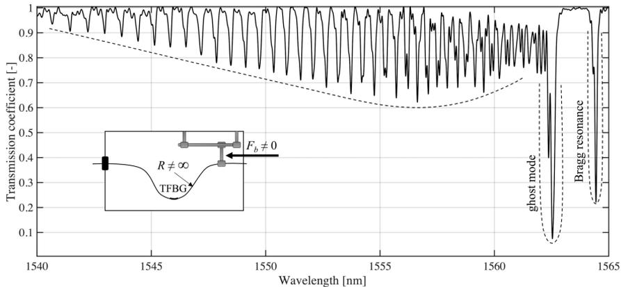
Fig. 4. Spectral characteristics of a bent TFBG measured in the transmission mode.
