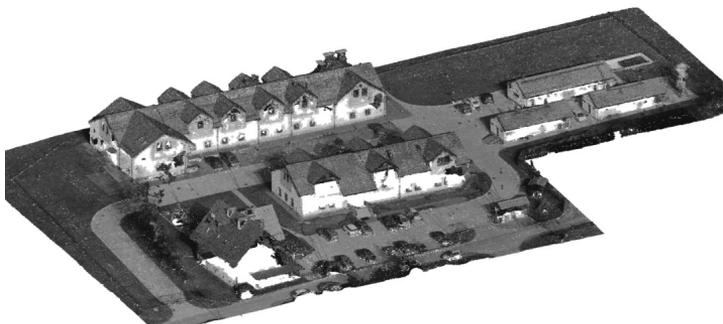
Fig. 5. Point cloud – derived from UAV photos
