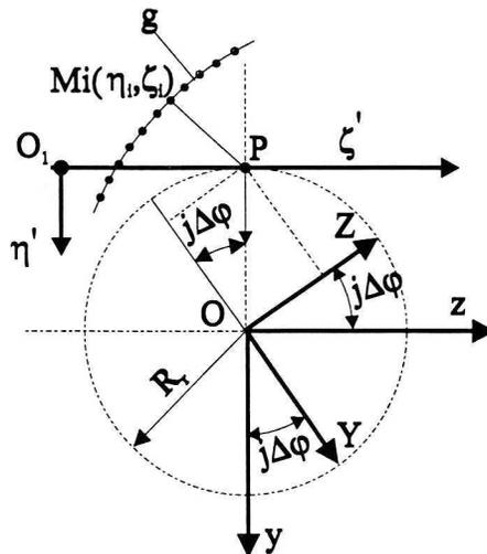
Fig. 6. Coordinates of the meshing pole P
