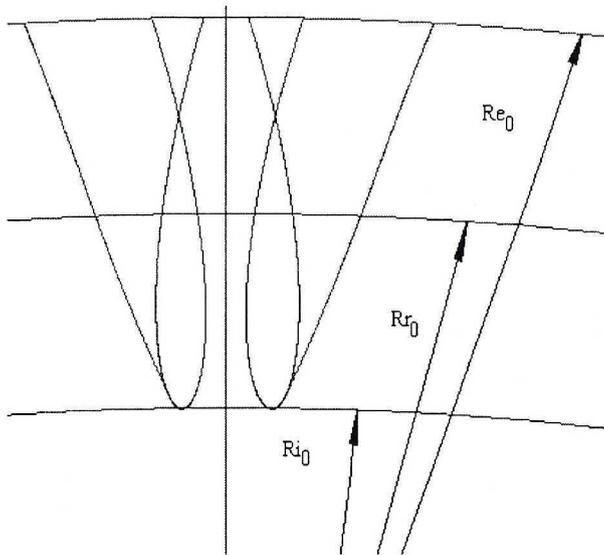
Fig. 7. Profile of the worm-gear tooth in the sectional plane  $H_0$
