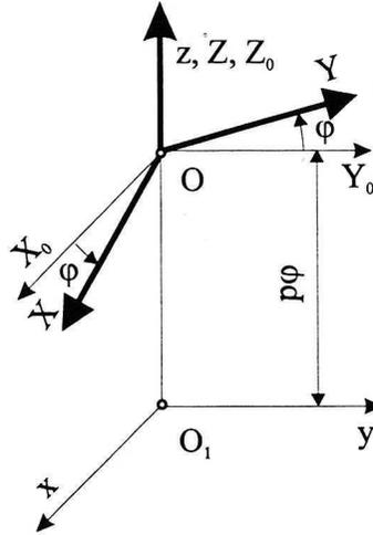
Fig. 3. Coordinate system used for the helical motion
