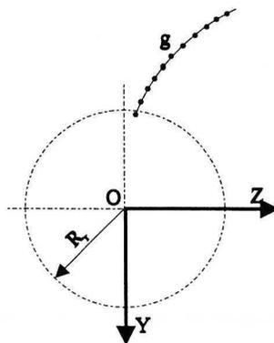
Fig. 9. Coordinate system ed for the profile of the worm-gear tooth
