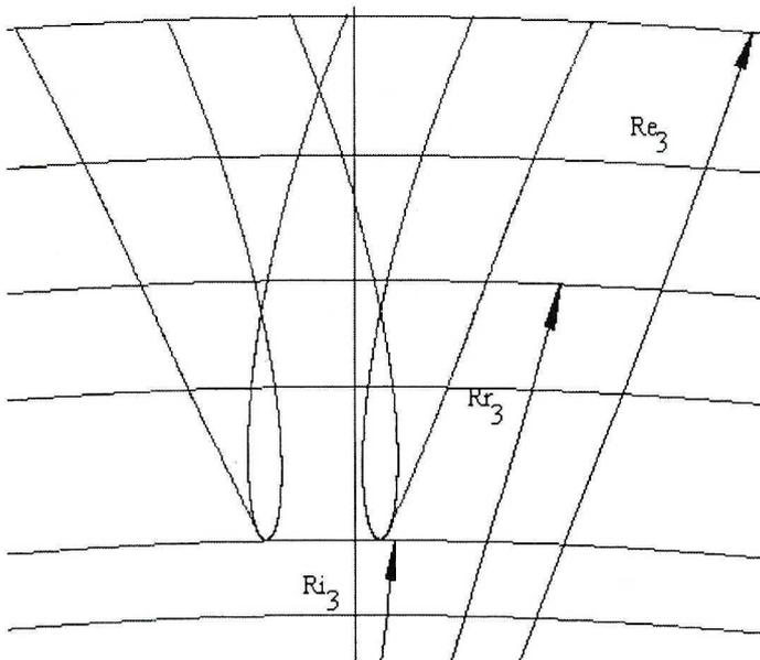
Fig. 8. Profile of the worm-gear tooth in the sectional plane  $H_3$
