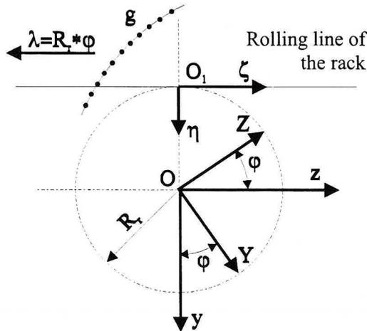
Fig. 5. Worm-gear flank generation
