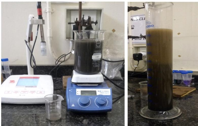
Fig. 3. Slurry preparation setup and settling test setup
