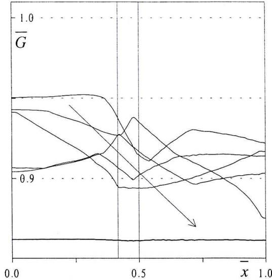
Fig. 10. Mass flow rate distribution at  $t = 0.2$  ms,  $t = 0.25$  ms,  $t = 0.3$  ms,  $t = 0.35$  ms,  $t = 0.4$  ms, and  $t = 2$  ms (thicker line). The arrow shows the development in time
