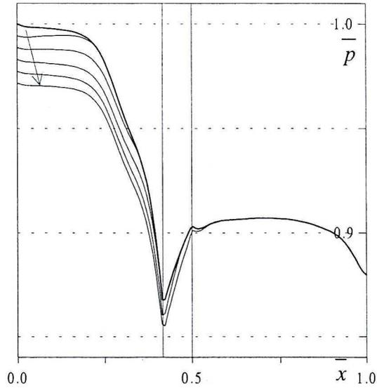
Fig. 2. Static pressure distribution at  $t=0$  (thicker line),  $t=0.02$  ms,  $t=0.04$  ms,  $t=0.06$  ms,  $t=0.08$  ms, and  $t=0.1$  ms. The arrow shows the development in time
