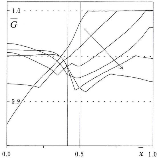
Fig. 9. Mass flow rate distribution at  $t=0.1$  ms,  $t=0.12$  ms,  $t=0.14$  ms,  $t=0.16$  ms,  $t=0.18$  ms, and  $t=0.2$  ms. The arrow shows the development in time
