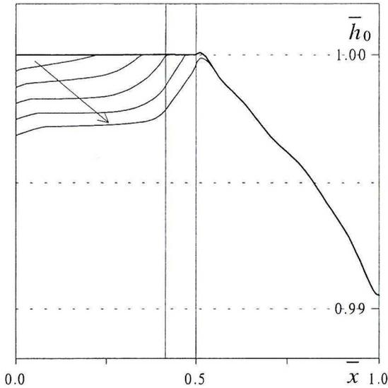
Fig. 5. Specific stagnation enthalpy distribution at  $t = 0$  (thicker line),  $t = 0.02$  ms,  $t = 0.04$  ms,  $t = 0.06$  ms,  $t = 0.08$  ms, and  $t = 0.1$  ms. The arrow shows the development in time
