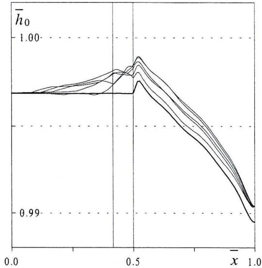
Fig. 7. Specific stagnation enthalpy distribution at  $t = 0.2$  ms,  $t = 0.25$  ms,  $t = 0.3$  ms,  $t = 0.35$  ms,  $t = 0.4$  ms, and  $t = 2$  ms (thicker line)
