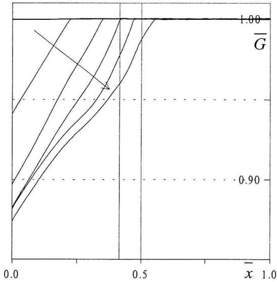
Fig. 8. Mass flow rate distribution at  $t=0$  (thicker line),  $t=0.02$  ms,  $t=0.04$  ms,  $t=0.06$  ms,  $t=0.08$  ms, and  $t=0.1$  ms. The arrow shows the development in time
