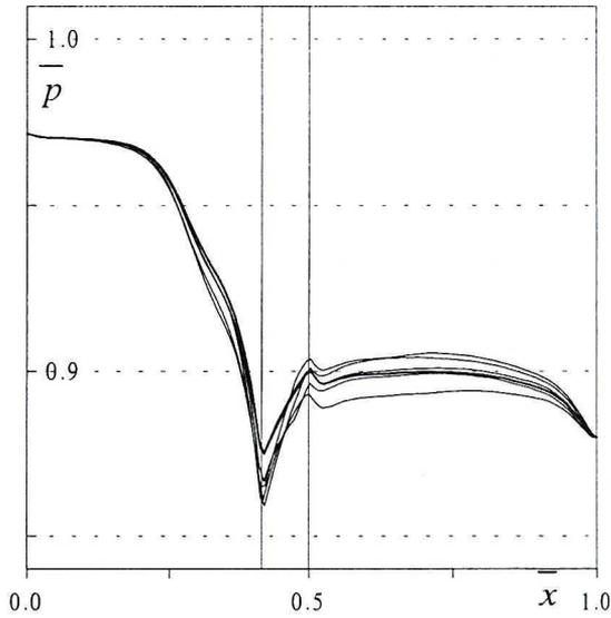
Fig. 4. Static pressure distribution at  $t = 0.2$  ms,  $t = 0.25$  ms,  $t = 0.3$  ms,  $t = 0.35$  ms,  $t = 0.4$  ms, and  $t = 2$  ms (thicker line)
