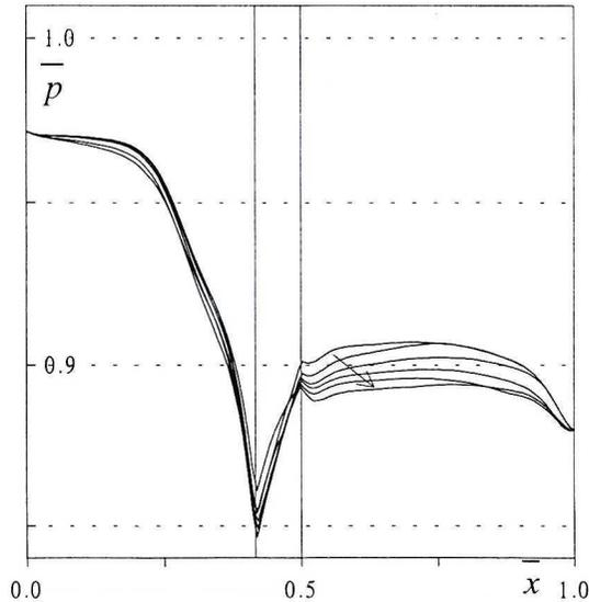
Fig. 3. Static pressure distribution at  $t=0.1$  ms,  $t=0.12$  ms,  $t=0.14$  ms,  $t=0.16$  ms,  $t=0.18$  ms, and  $t=0.2$  ms. The arrow shows the development in time
