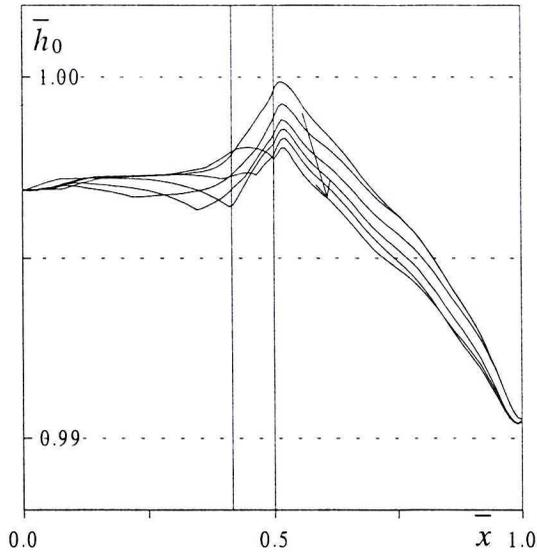
Fig. 6. Specific stagnation enthalpy distribution at  $t = 0.1$  ms,  $t = 0.12$  ms,  $t = 0.14$  ms,  $t = 0.16$  ms,  $t = 0.18$  ms, and  $t = 0.2$  ms. The arrow shows the development in time
