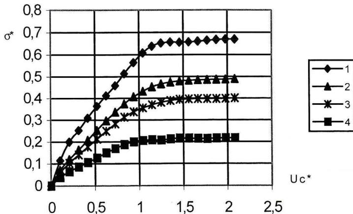
Fig. 4. Load-shortening curves for plates „III”: 1 –  $g/h=0$ ; 2 –  $g/h=0.4$ ; 3 –  $g/h=0.6$ ; 4 –  $g/h=1.0$
