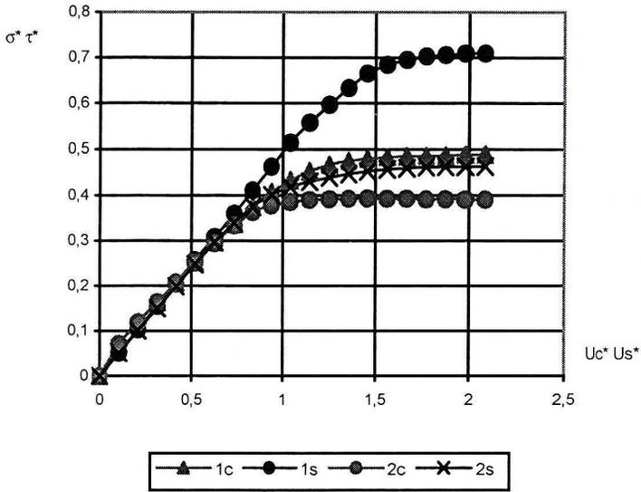
Fig. 8. Load-displacement curves for three layered plates ( $g/h=0.4$ ); 1c – pure compression; 1s – pure shear; 2c, 2s – combined loading;  $\Delta U_c^*/\Delta U_s^*=1$
