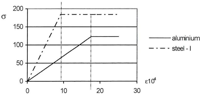
Fig. 5b. Material stress-strain relations for plates "I"
