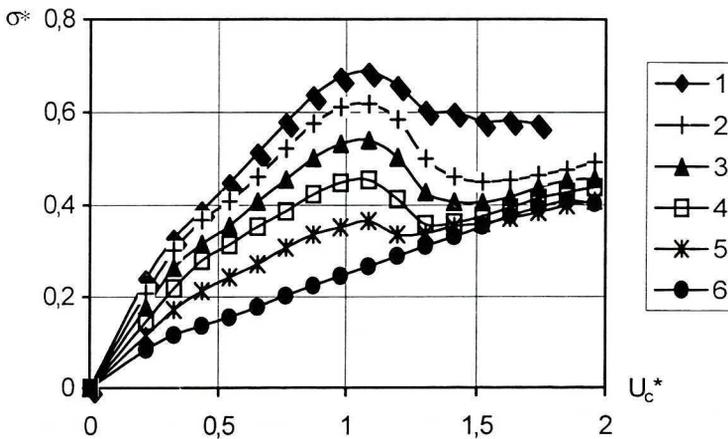
Fig. 2. Load versus shortening curves for plates „I”: 1 –  $g/h=0$ ; 2 –  $g/h=0.2$ ; 3 –  $g/h=0.4$ ; 4 –  $g/h=0.6$ ; 5 –  $g/h=0.8$ ; 6 –  $g/h=1.0$
