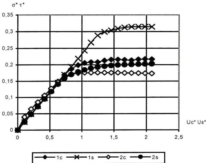
Fig. 9. Load-displacement curves for aluminium plates ( $g/h=1.0$ ); 1c – pure compression; 1s – pure shear; 2c, 2s – combined loading;  $\Delta U_c^*/\Delta U_s^*=1$
