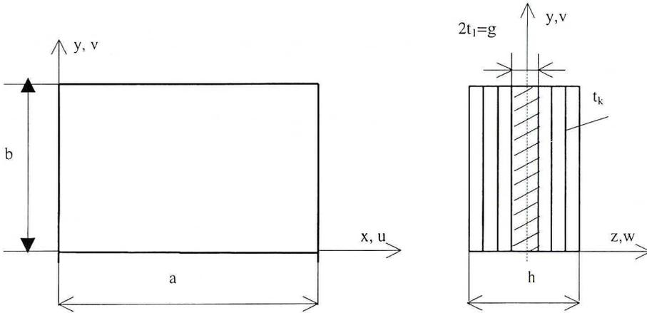
Fig. 1b. Geometry of a plate
