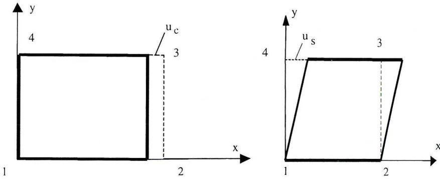
Fig. 1a. Rectangular plates subjected to compression and shear
