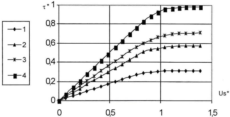
Fig. 6. Average shear stress versus angle of rotation for plates subjected to pure shear; 1 –  $g/h=0$ ; 2 –  $g/h=0.4$ ; 3 –  $g/h=0.6$ ; 4 –  $g/h=1.0$
