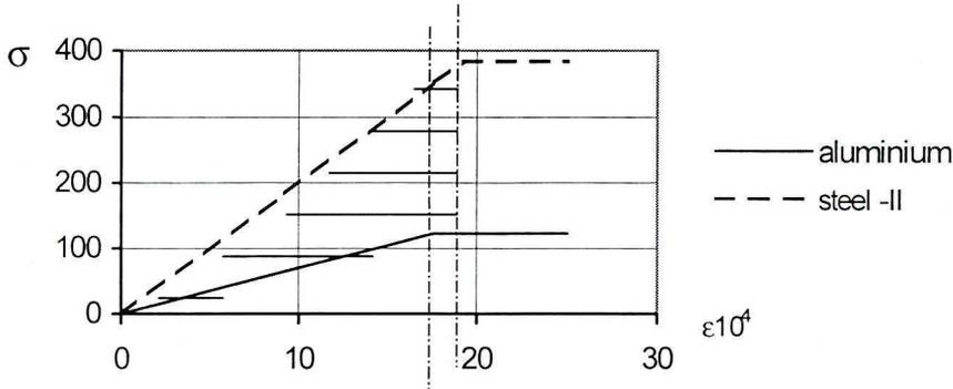
Fig. 5a. Material stress-strain relations for plates "II" and "III"
