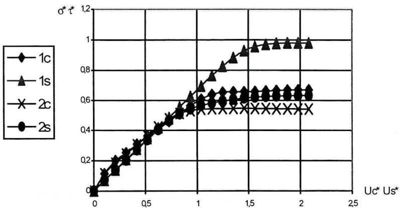
Fig. 7. Load-displacement curves for steel plates ( $g/h=0$ ); 1c – pure compression; 1s – pure shear; 2c, 2s – combined loading;  $\Delta U_c^*/\Delta U_s^*=1$
