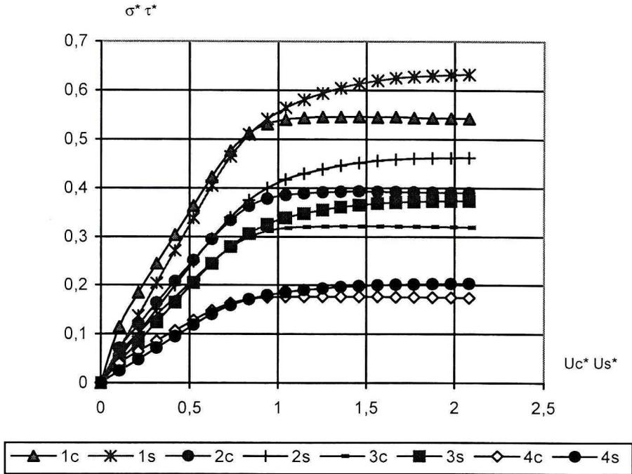
Fig. 10. Load-displacement curves for plates subjected to combined loading; 1 –  $g/h=0$ ; 2 –  $g/h=0.4$ ; 3 –  $g/h=0.6$ ; 4 –  $g/h=1.0$ ; (c – compression, s – shear),  $\Delta U_c^*/\Delta U_s^*=1$
