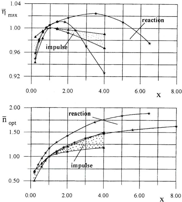
Fig.11 Comparison of courses of the maximum efficiencies and the optimum relative rotational speed for impulse and reaction type groups tested
