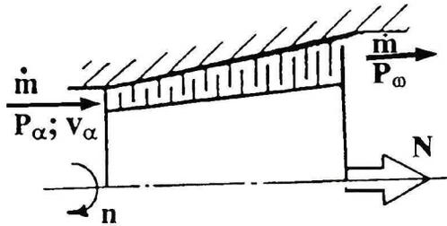
Fig. 1 Scheme of turbine stage group
