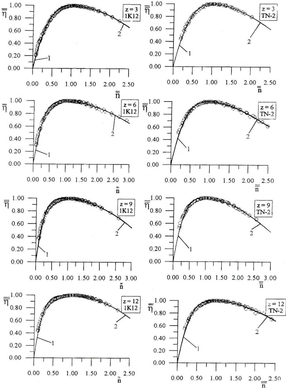
Fig. 8 Efficiency characteristics of the tested stage groups in the form  $\eta = \eta(n)$  ;
