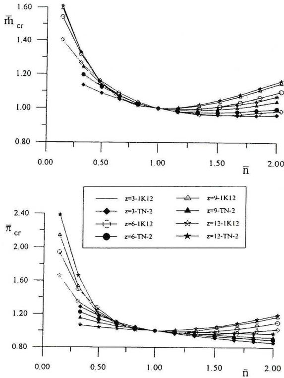
Fig. 5. Relative critical mass flow rate - coefficient  $A(\bar{n})$  and relative critical pressure ratio - coefficient  $B(\bar{n})$  as a function of the rotational speed and the number of stages in the group for the 1K12 and TN-2 groups
