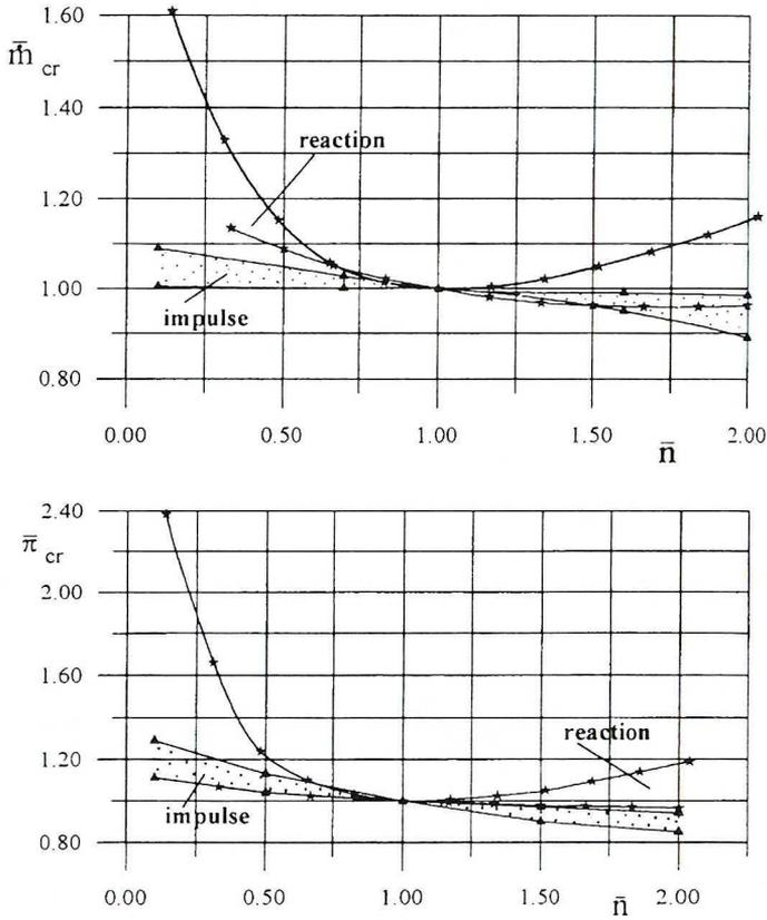
Fig.10 Comparison of courses of the relative critical mass flow rates and the relative critical pressure ratio for impulse and reaction type groups tested
