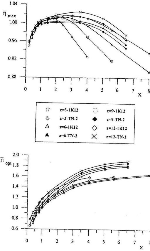
Fig. 9 Maximum efficiencies and optimum relative rotational speed as functions of the pressure ratio indicator  $X$  and the number of stages in the group for the 1K12 and TN-2 groups
