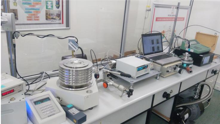
Fig. 3. Cross-floating and digital manometer-assisted calibration setup.
