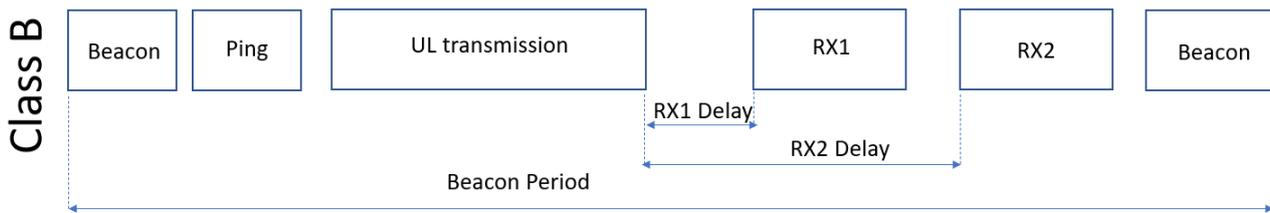
Fig. 5. Devices classes - Class B [own work based on: [82, 90, 91]]
