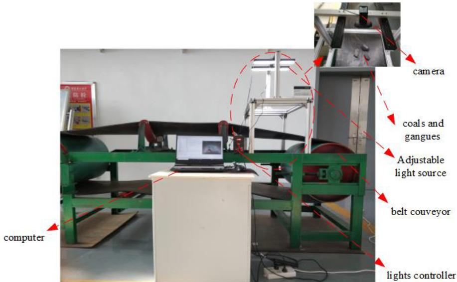
Fig. 7. Coal and gangue identification and location device
