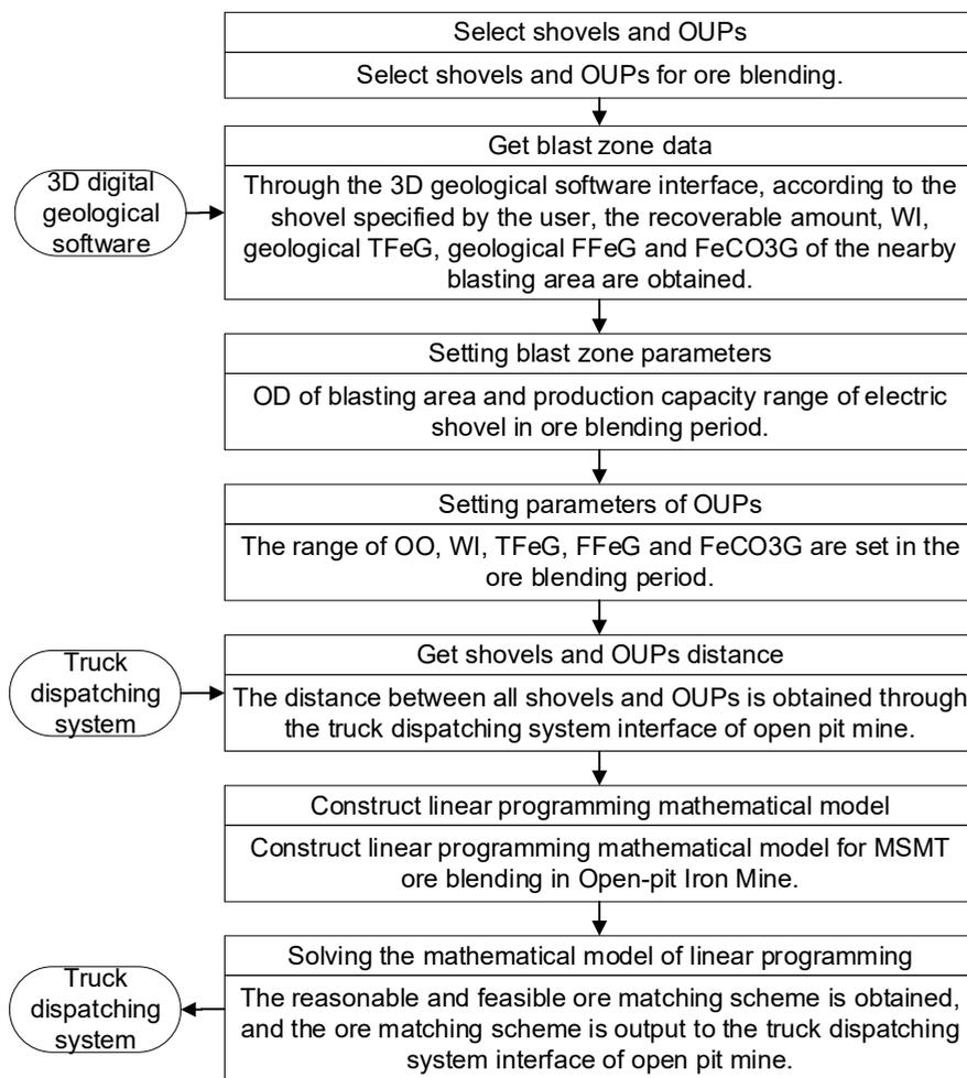
Fig. 1. Schematic diagram of ore blending process
