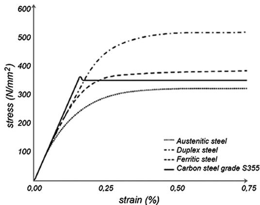
Fig. 6. Stress-strain curves of stainless and carbon steels
