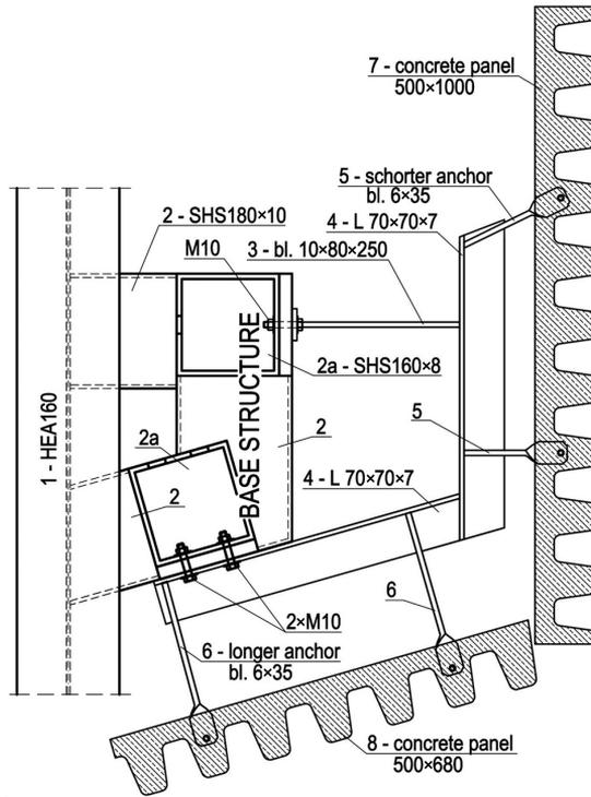
Fig. 2. Schematic representation of the tested mock-up
