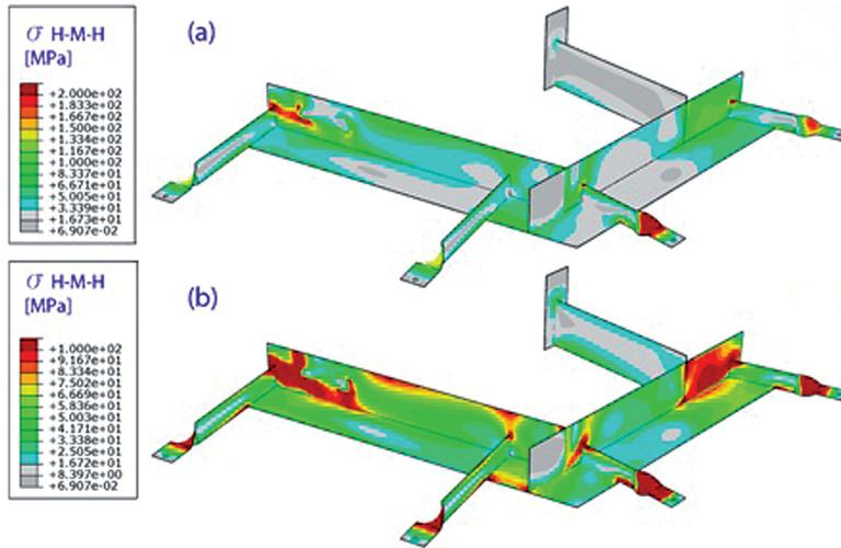
Fig. 14. Contour maps of von Mises equivalent stresses. Two different colour scales were applied
