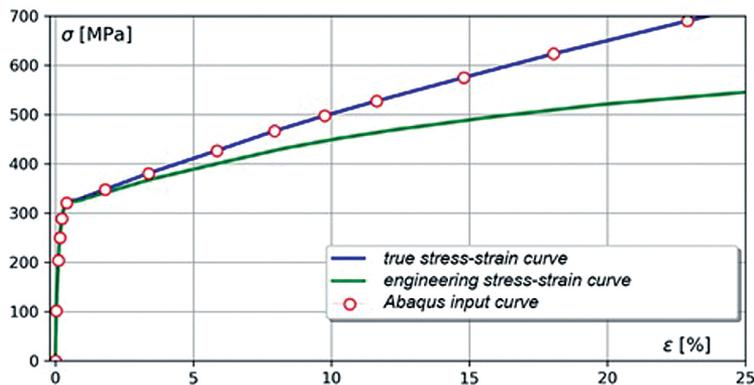
Fig. 10. Averaged stress-strain curves for steel grade 1.4301
