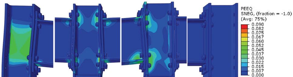
Fig. 15. Map of strains of joint (from left W13 to W16) with 15 mm thickness extended end-plate at level of structure +10.50 at 8<sup>th</sup> second of analysis
