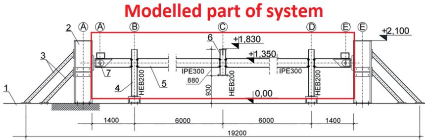
Fig. 2. Planar view of frame substructure tested in [12, 19]
