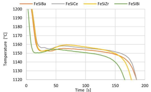
Fig. 13. Cooling curves for ductile cast iron after inoculation with various inoculants
