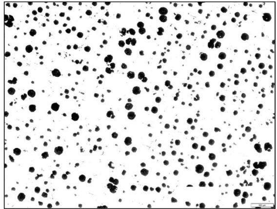
Fig. 4. Image of the cast iron microstructure, 299 graphite precipitates per  $mm^2$ ,  $T_{e_{min}}$  1155°C
