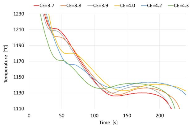
Fig. 5. Cooling curves for variable value of carbon equivalent (CE)
