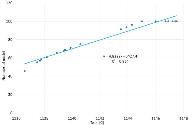
Fig. 1. Number of nuclei as a function of  $T_{e_{min}}$  temperature (values derived from DTA curves)
