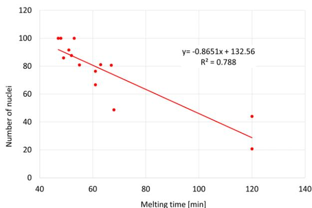
Fig. 9. Effect of melting time on the number of nuclei
