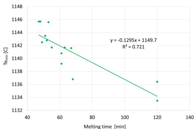
Fig. 8. Effect of melting time on the minimum eutectic temperature ( $T_{\text{min}}$ )
