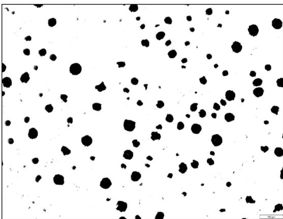
Fig. 3. Image of the cast iron microstructure, 109 graphite precipitates per  $mm^2$ ,  $T_{e_{min}}$  1143°C
