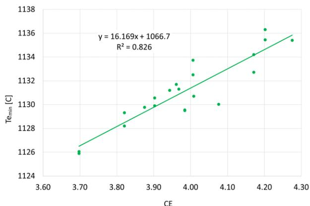
Fig. 6. Minimum eutectic temperature ( $T_{\text{min}}$ ) as a function of carbon equivalent (CE)
