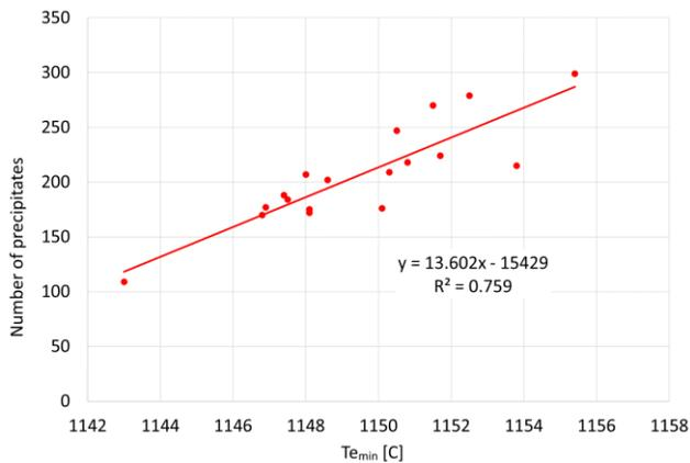
Fig. 2. Number of graphite precipitates in ductile cast iron, obtained in metallographic tests as a function of  $T_{e_{min}}$  temperature
