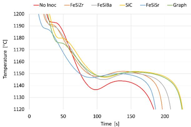
Fig. 10. Cooling curves without and after primary inoculation
