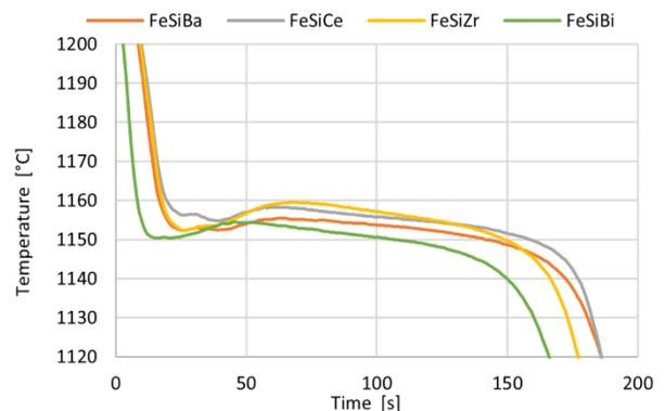
Fig. 14. Minimum eutectic temperature ( $T_{\min}$ ) after the introduction of different inoculants in the secondary inoculation process
