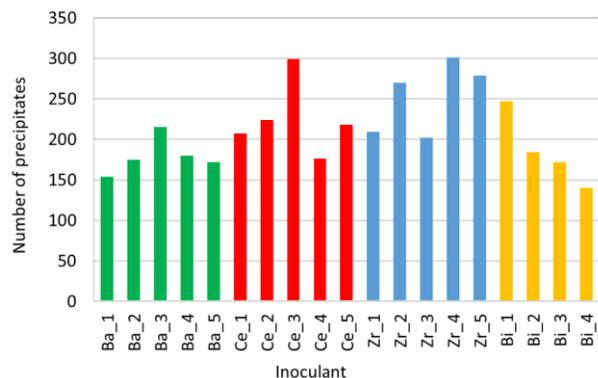
Fig. 15. Effect of secondary inoculation and inoculant used on the number of graphite precipitates in ductile cast iron
