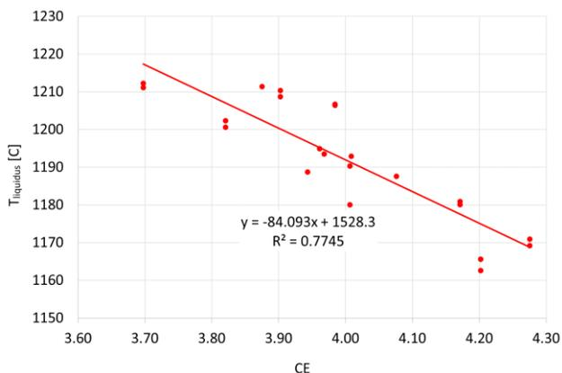
Fig. 7.  $T_{\text{liquidus}}$  temperature as a function of carbon equivalent (CE)
