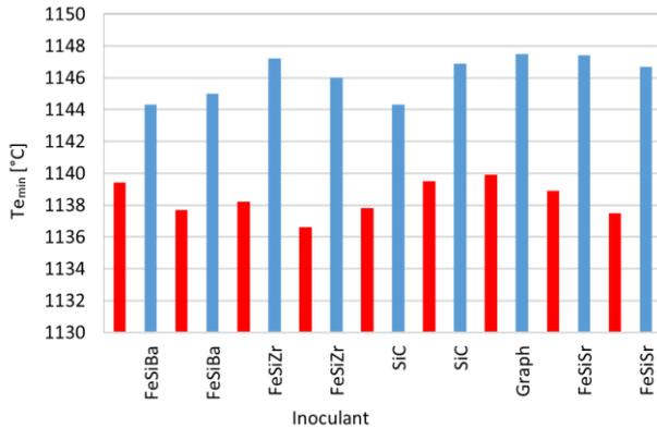
Fig. 11. Minimum eutectic temperature ( $T_{\min}$ ) after the introduction of different inoculants
