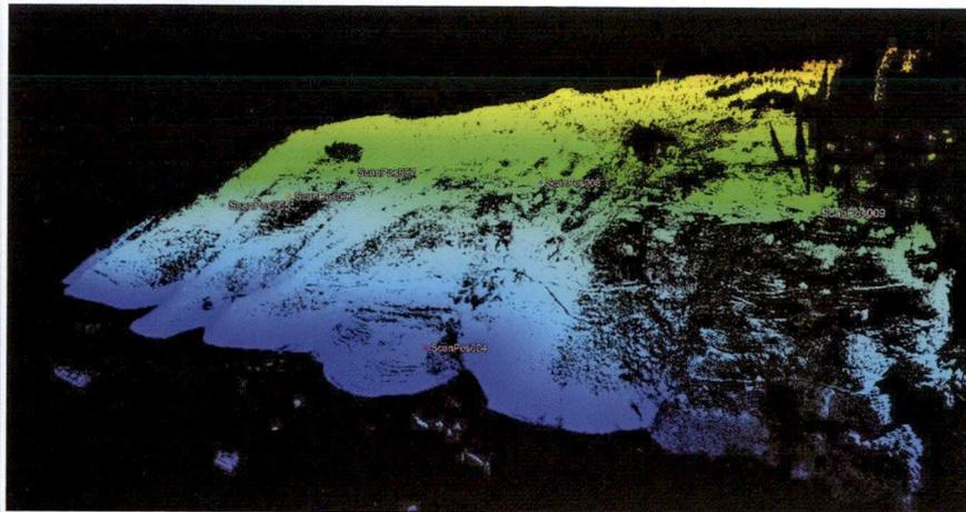
Results of terrestrial scanning of the Shuping landslide – a cloud of altitude data
