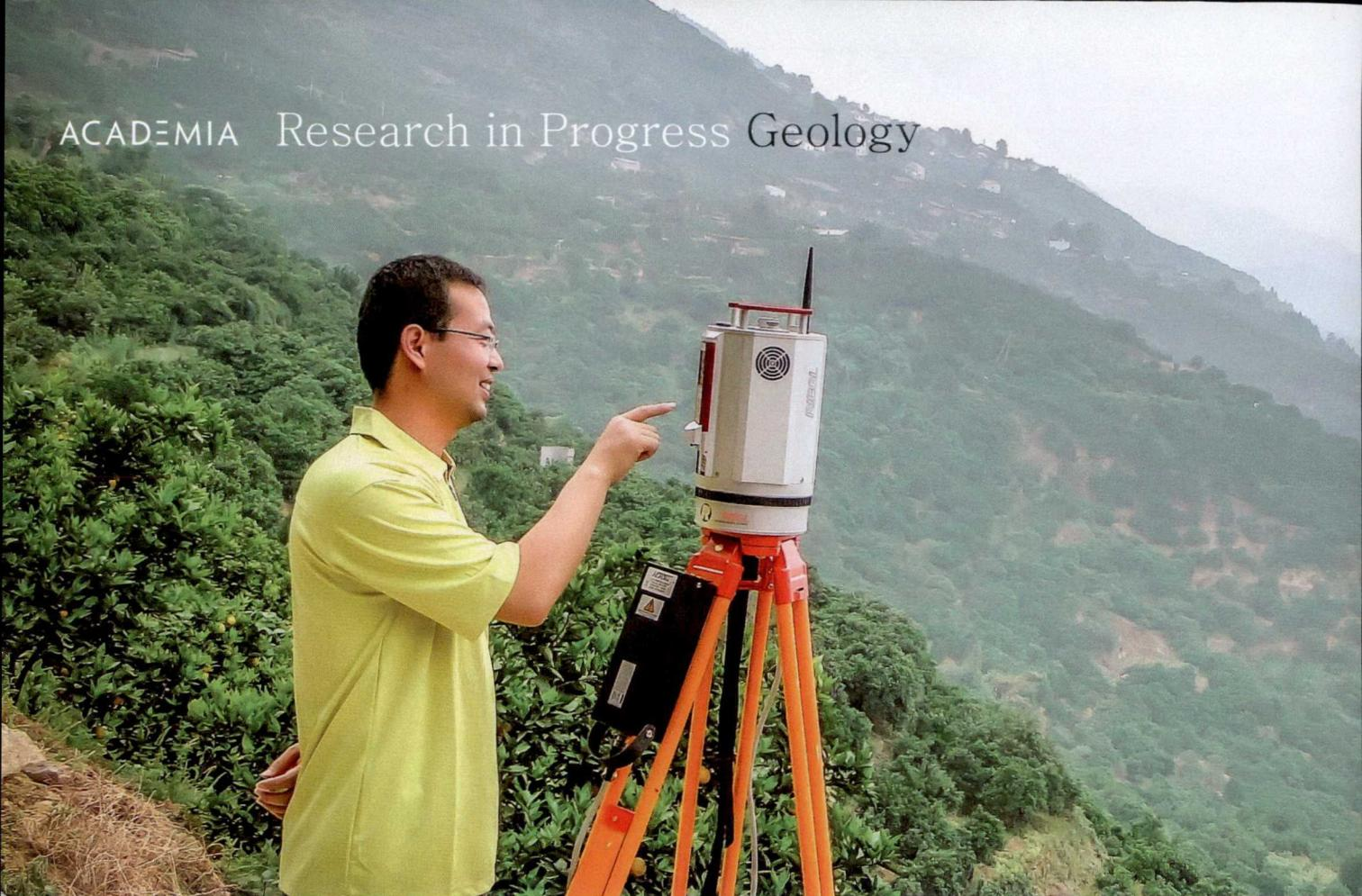
Scanning the Shuping landslide – Dr. Fan Jinghui sets the parameters of a laser scanner
