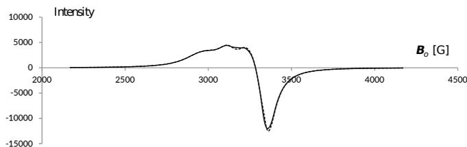
**Fig. 4.** EPR resonance spectra for loose nanomaterial composed of hydrated copper sulfate, for two directions  $(i) = x, y$  of magnetic field  $B_0$  defined by Fig. 3.  $(i) = x$  – solid line,  $(i) = y$  – dashed line
