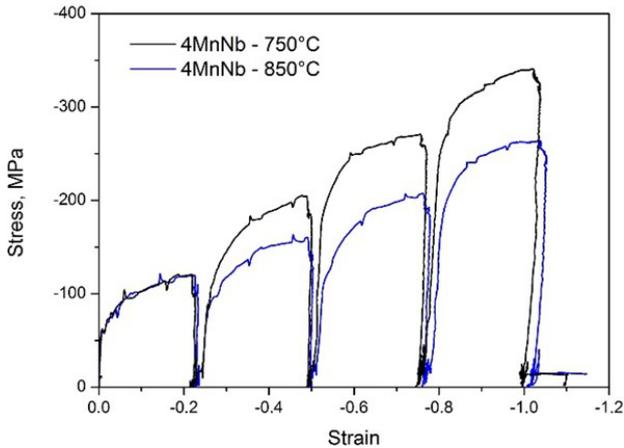
**Fig. 2.** Effect of final deformation temperature on  $\sigma - \varepsilon$  curves of 4MnNb steel
