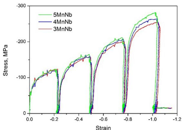
**Fig. 1.** Effect of Mn addition on the  $\sigma$ - $\epsilon$  curves in the four-step compression test of the tested steels
