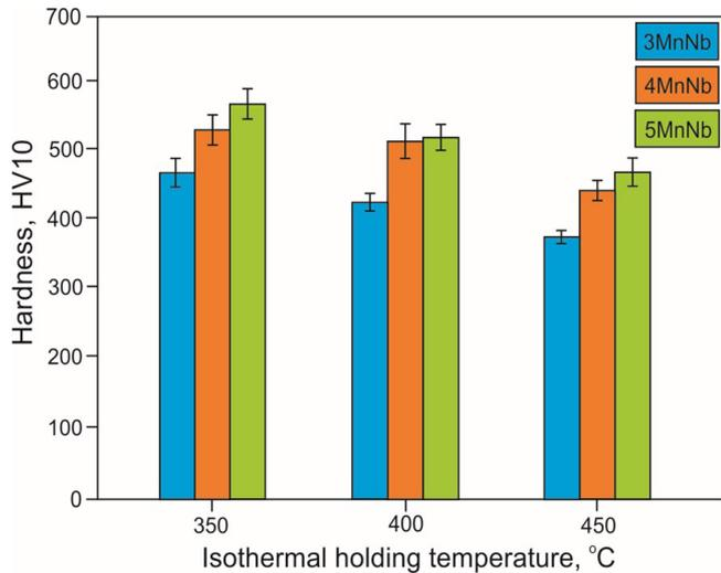
**Fig. 9.** Effect of isothermal holding temperature on hardness of the tested steels
