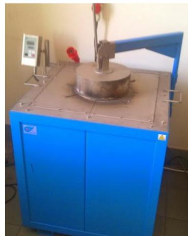
Fig. 7. General view of the PT 40/1300 resistance pit furnace
