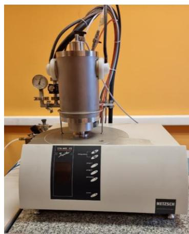
Fig. 5. Overview of the STA 449 F3 Jupiter thermal analyzer
