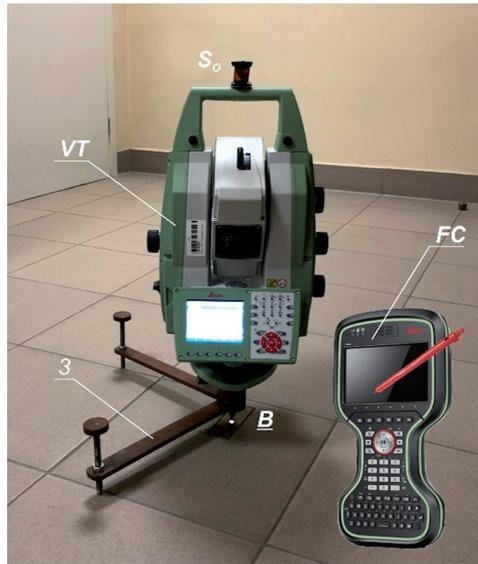
Fig. 3. View of a scan station Leica MS50 with additional equipment and a remote controller Leica CS20 located on a standpoint (*VT* – video total station/scan station; *FC* – functional remote controller, *3* – mini-tripod; *S<sub>O</sub>* – orienting prism/signal; *B* – base point)
