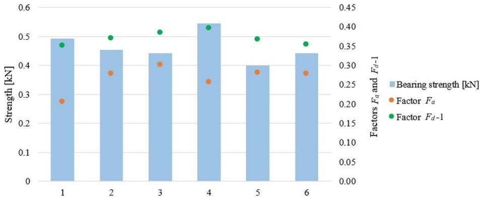
Fig. 12. Comparison of average values of bearing strength and delamination factors  $F_a$  and  $F_d$  for holes made by different drills: plain HSS (drill 1), HSS with 5% addition of cobalt, (drill 2), HSS with 5% addition of cobalt with titanium coating (drill 3), HSS with titanium coating (drill 4), cemented carbide (drill 5) and HSS tipped with tungsten carbide (drill 6)
