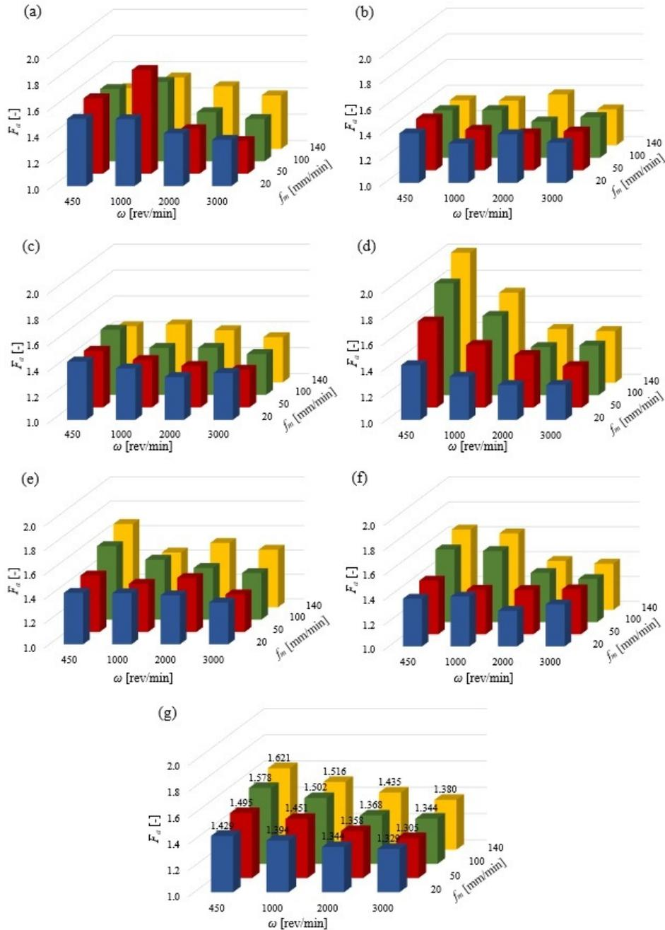
Fig. 8. Delamination factor  $F_d$  for holes made by different drills: (a) plain HSS (drill 1), (b) HSS with 5% addition of cobalt (drill 2), (c) HSS with 5% addition of cobalt with titanium coating (drill 3), (d) HSS with titanium coating (drill 4), (e) cemented carbide (drill 5), (f) HSS tipped with tungsten carbide (drill 6) and (g) factor averaged for all drills
