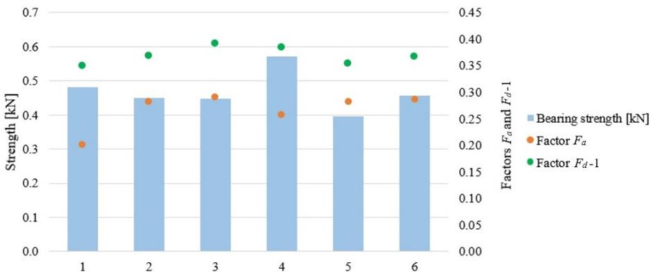
Fig. 13. Comparison of medians of bearing strength and delamination factors  $F_a$  and  $F_d$  for holes made by different drills: plain HSS (drill 1), HSS with 5% addition of cobalt (drill 2), HSS with 5% addition of cobalt with titanium coating (drill 3), HSS with titanium coating (drill 4), cemented carbide (drill 5) and HSS tipped with tungsten carbide (drill 6)
