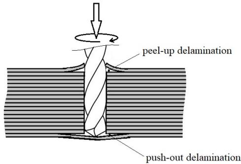
Fig. 4. Peel-up and push-out delamination
