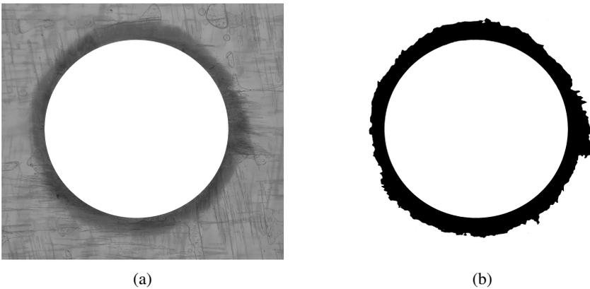
Fig. 5. (a) Exemplary raw picture of a hole; (b) The picture after processing
