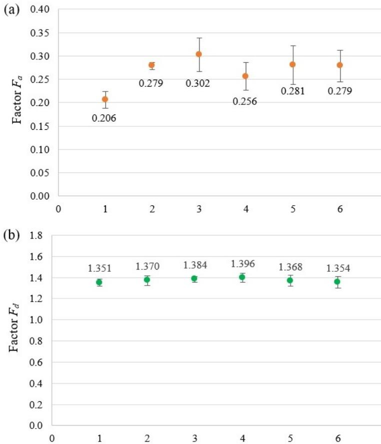
Fig. 11. Delamination factors (a)  $F_a$  and (b)  $F_d$  for holes made by different drills: plain HSS (drill 1), HSS with 5% addition of cobalt, (drill 2), HSS with 5% addition of cobalt with titanium coating (drill 3), HSS with titanium coating (drill 4), cemented carbide (drill 5) and HSS tipped with tungsten carbide (drill 6)
