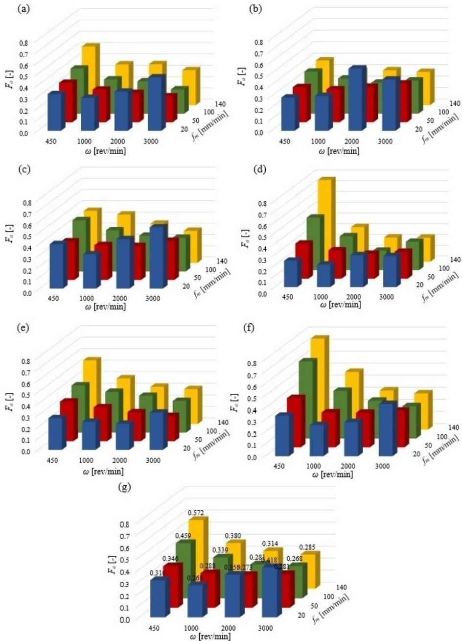
Fig. 7. Delamination factor  $F_a$  for holes made by different drills: (a) plain HSS (drill 1), (b) HSS with 5% addition of cobalt (drill 2), (c) HSS with 5% addition of cobalt with titanium coating (drill 3), (d) HSS with titanium coating (drill 4), (e) cemented carbide (drill 5), (f) HSS tipped with tungsten carbide (drill 6) and (g) factor averaged for all drills
