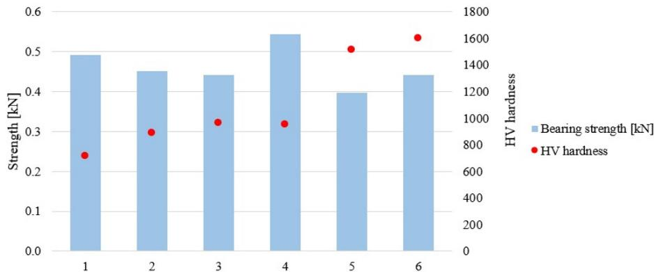
Fig. 14. Comparison of average values of bearing strength and the HV hardness of different drills: plain HSS (drill 1), HSS with 5% addition of cobalt, (drill 2), HSS with 5% addition of cobalt with titanium coating (drill 3), HSS with titanium coating (drill 4), cemented carbide (drill 5) and HSS tipped with tungsten carbide (drill 6)
