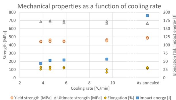
Fig. 6. Mechanical properties as a function of cooling rate of cast duplex steel Gr4A
