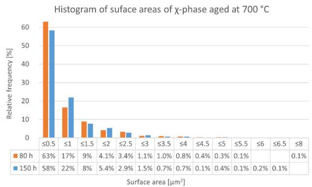
Fig. 4. Histogram of the surface area of  $\chi$ -phase after ageing at 700 °C at different times in Gr 4A steel
