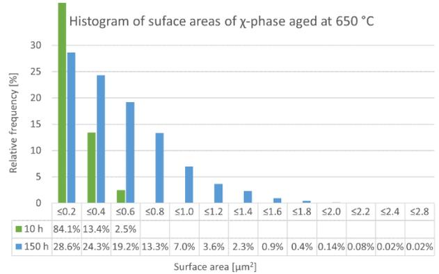
Fig. 3. Histogram of the surface area of  $\chi$ -phase after ageing at 650 °C at different times in Gr 4A steel
