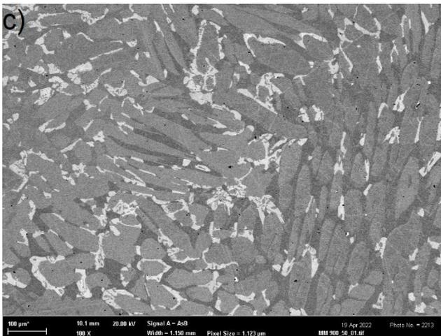
Fig. 2. SEM microstructure of Gr 4A steel after ageing at: (a) 800 °C/10 h (magnification 500x, bar 10 μm), (b) 800 °C/50 h (magnification 500x, bar 10 μm), (c) 900 °C/50 h (magnification 100x, bar 100 μm)
