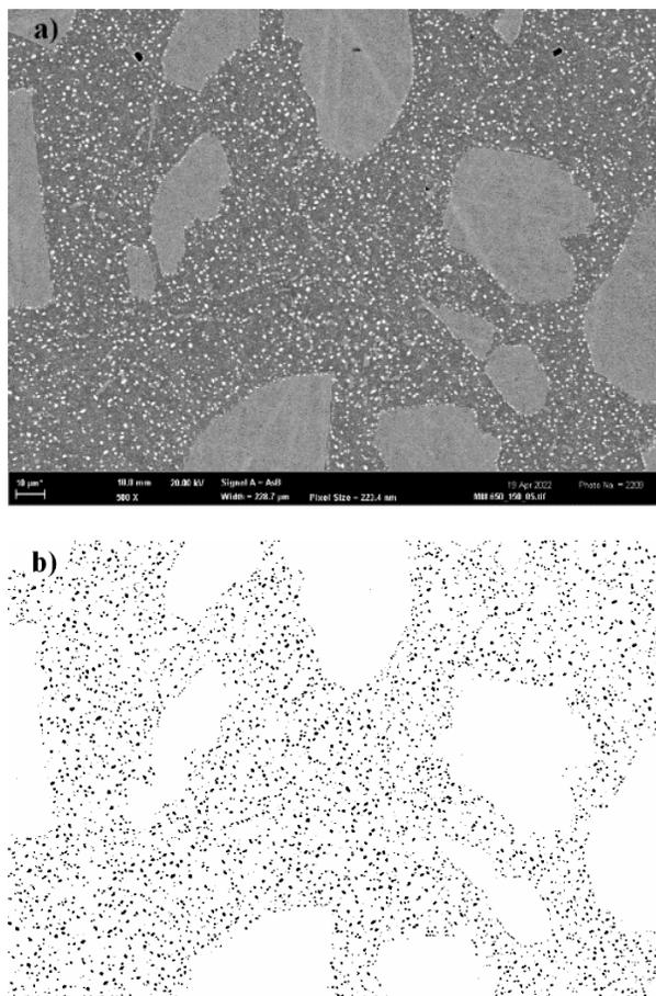
Fig. 1. Microstructure of the Gr 4A steel after 150 h of ageing at 650 °C (magnification 500x, bar 10 μm): a) original SEM image, b) thresholded image
