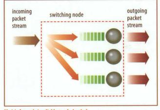
Model of a packet switching node (router)
