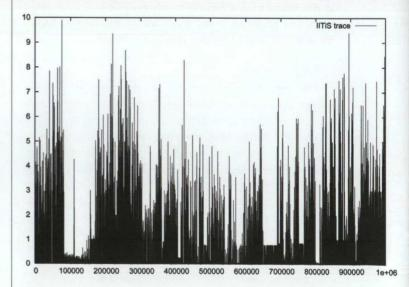
Changes in intensity of packet movement over time. Measurements taken at the PAS Institute of Theoretical and Applied Informatics; horizontal axis: packet number; vertical axis: time interval in seconds between packets
