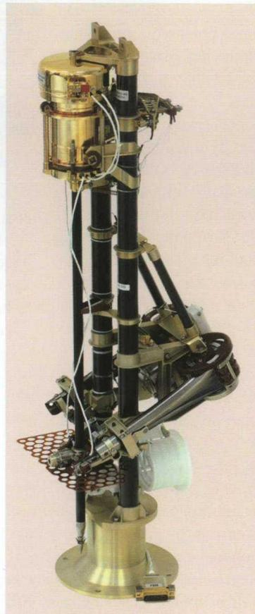
MUPUS Penetrator device, constructed at the PAS Space Research Centre for the Rosetta mission
