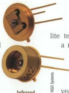
**Infrared detectors made by the Polish company VIGO Systems, taken to Mars on the Curiosity mission**
