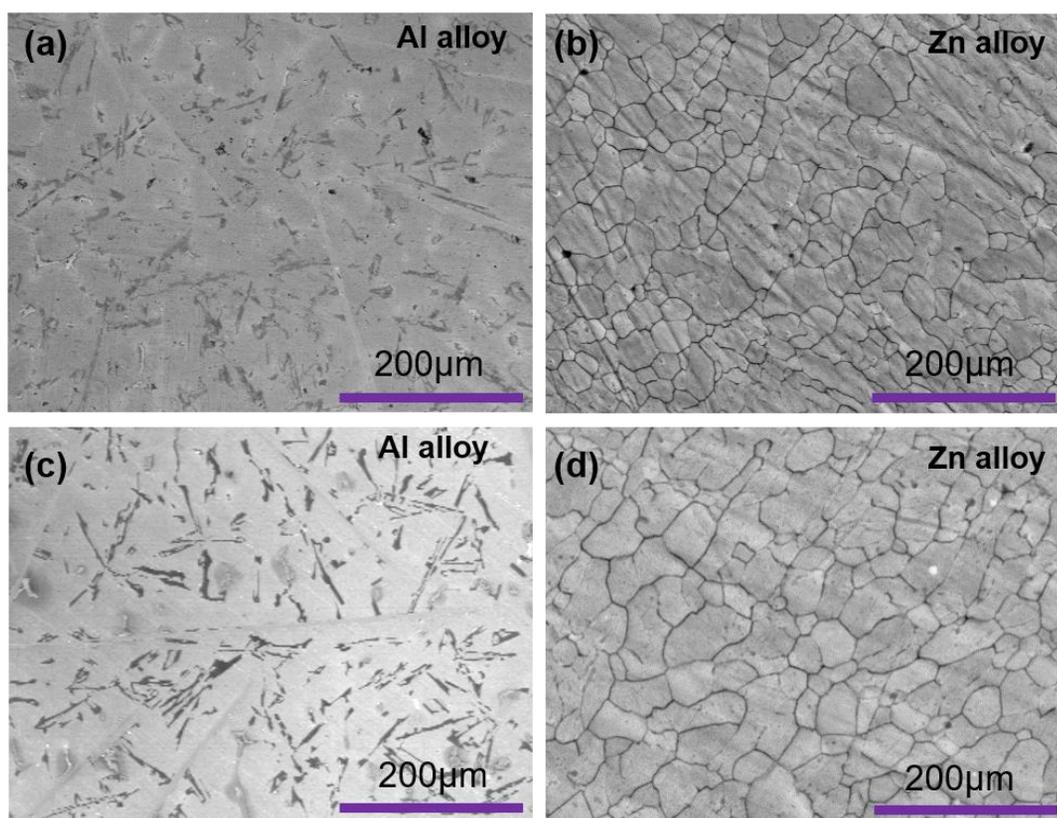
Fig. 7. Surface texture and microstructure of alloys using Brahmaputra River sand (a and b) and commercial silica foundry sand (c and d)
