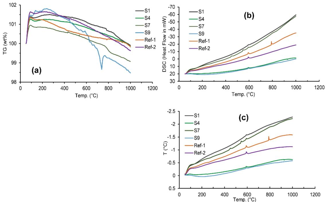
Fig. 5. Thermogravimetric and thermal analysis of sand specimen (a) TG, (b) DSC, (c)  $\Delta T$  curves
