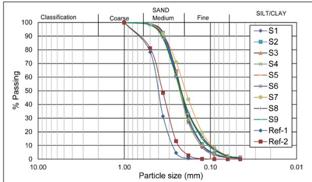
Fig. 4. Particle size distribution curves of sand specimen
