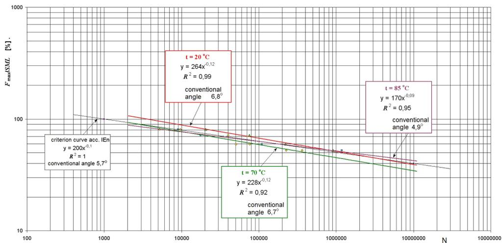
Fig. 7. Fatigue characteristics of composite insulators of manufacturer B, for the 220 kV (400 kV) lines, determined at different temperatures of lower end-fitting
