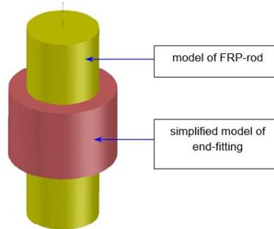
Fig. 8. Simplified presentation of essence of a composite insulator end-fitting structure
