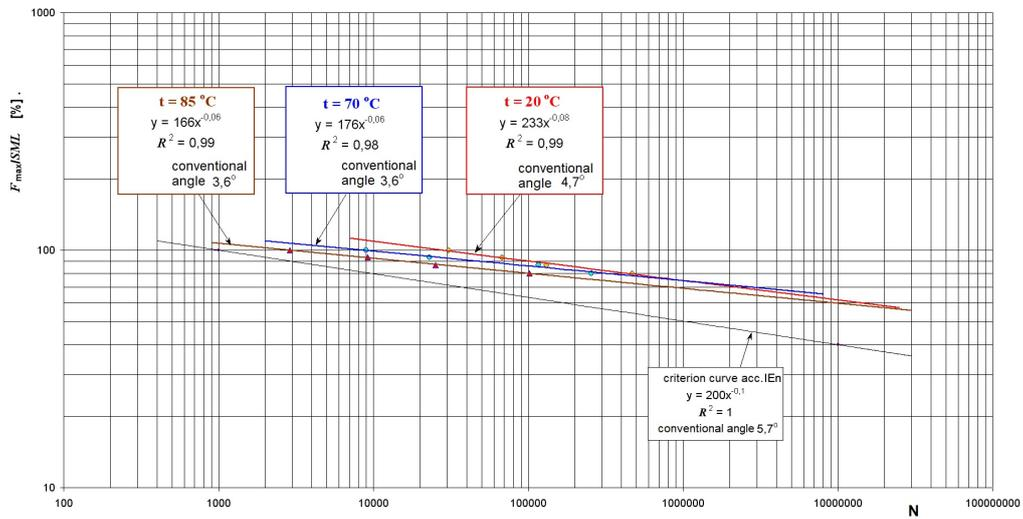
Fig. 6. Fatigue characteristics of composite insulators of manufacturer A, for the 220 kV (400 kV) lines, determined at different temperatures of lower end-fitting
