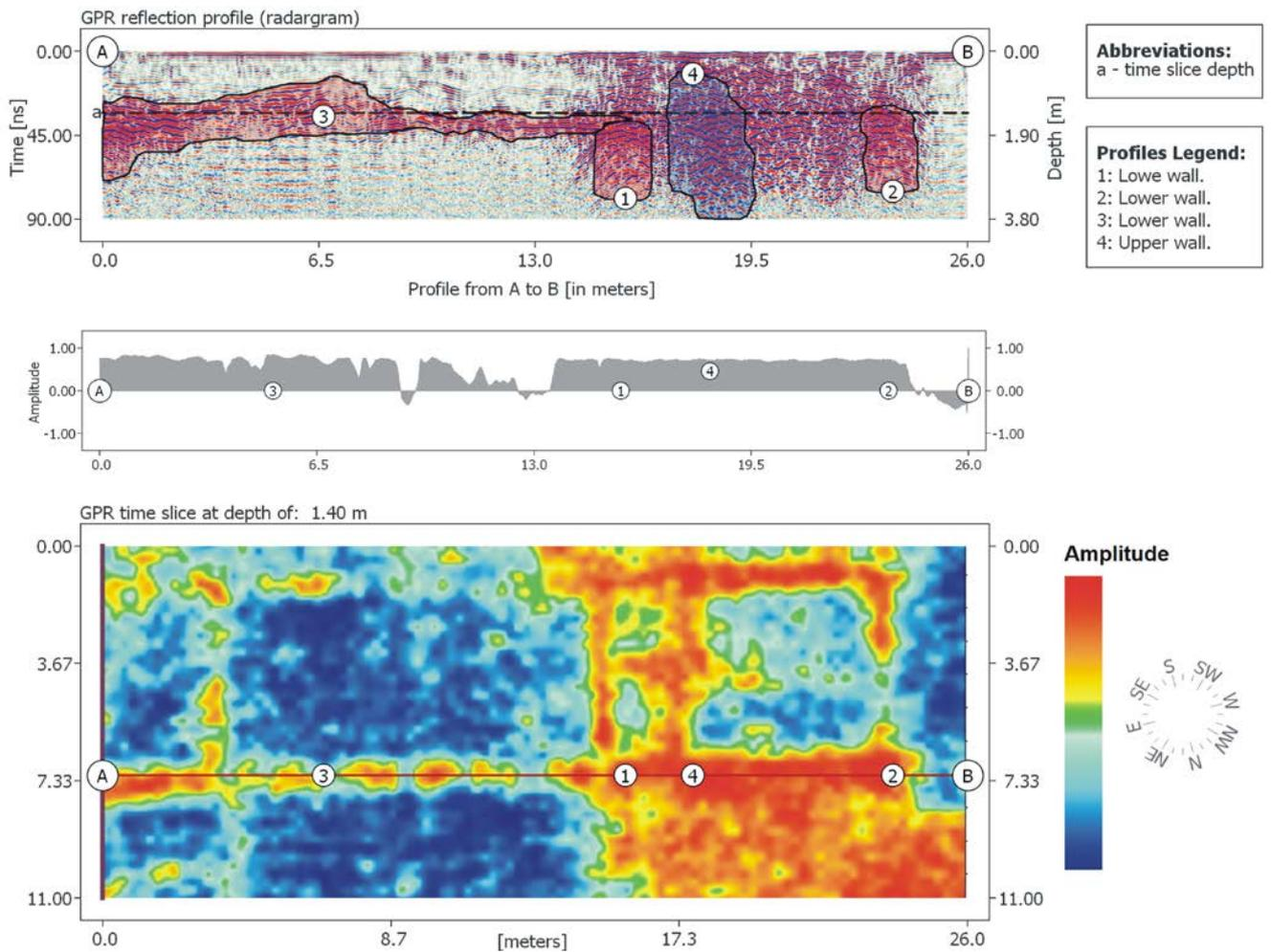
**Fig. 8.** GPR plan (time slice) prepared for a depth of approx. 1.4 m compiled with reflection profile no. 29, records of the relative amplitude value and interpretation (drawing and interpretation by F. Welc).
