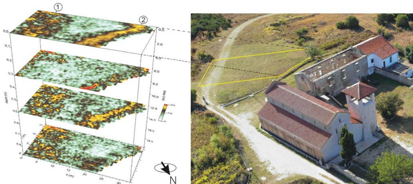
**Fig. 4.** Measurement area (right), selected GPR plans for individual depth levels. 1 – signal amplification zone corresponding to leveling embankments for the local road, 2 – analogous GPR signal amplification zone echoing the embankment resulting from the excavation of a modern drainage channel (drawing, processing and interpretation by F. Welc).
