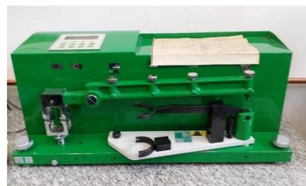
Fig. 2. Universal sand strength testing machine
