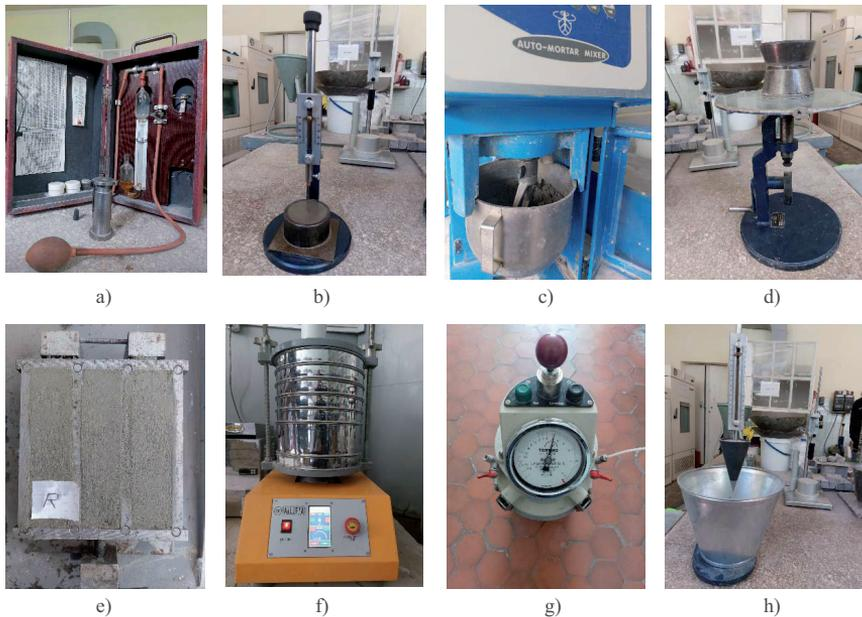
Fig. 1. Tovarov device (a), Vicat apparatus (b), mixer (c), flow table (d), 40×40×160 mm prism filled in with reference mortar (e), standard sieves (f), air content meter (g) and standard cone apparatus (h) were used to determine the properties of mortar and its constituents
