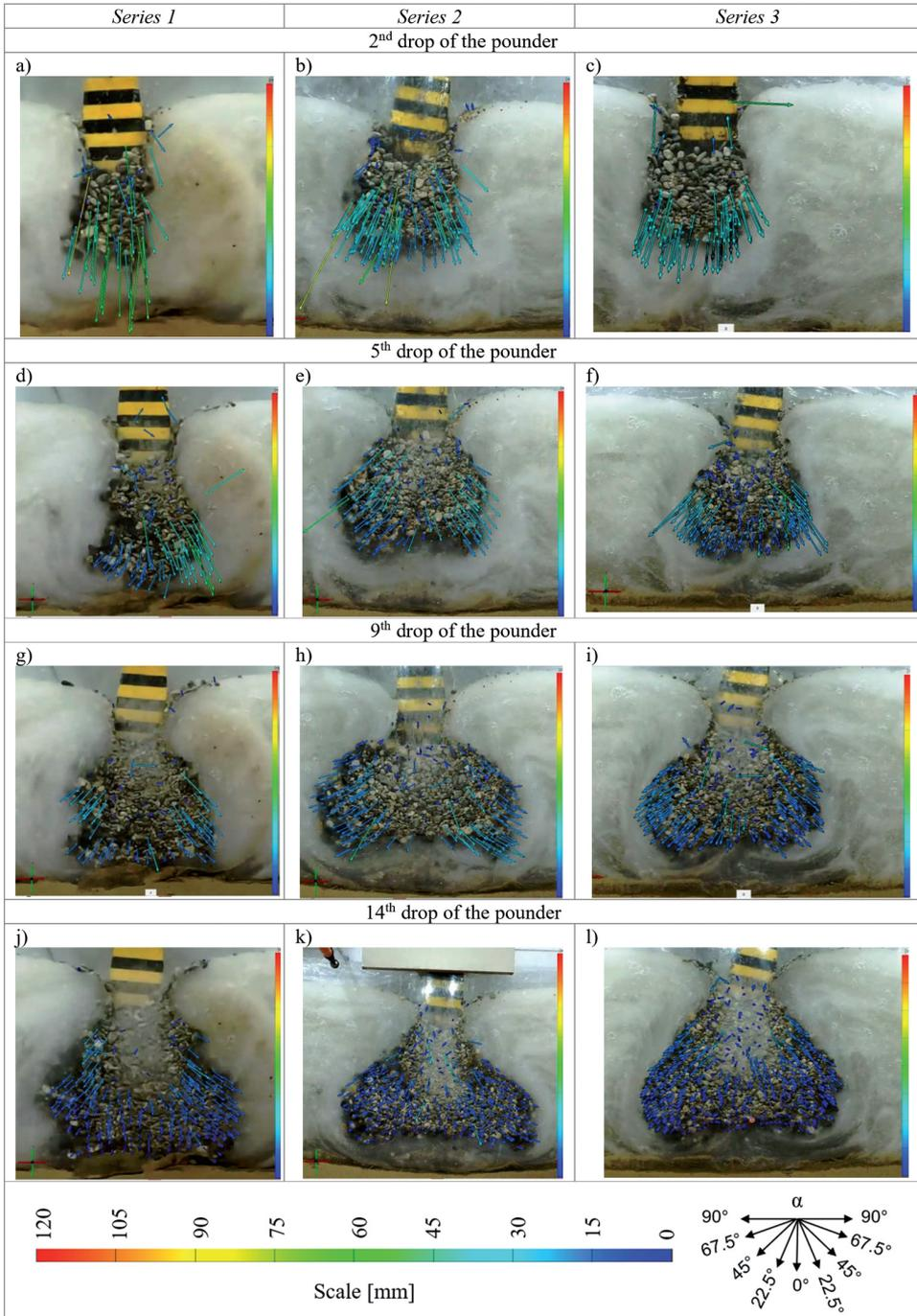
Fig. 7. The vectors of the resultant displacements of the backfill material – column B,  $H_s/H_p = 2.0$
